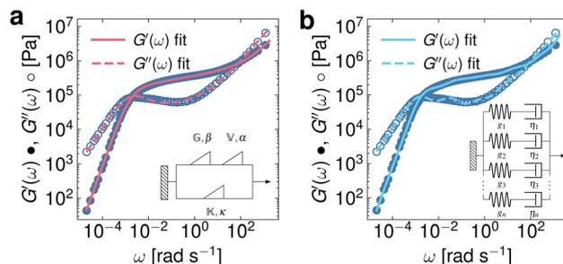
Fig. 4 Comparison between pyRheo and RepTate frameworks applied to describe the small amplitude oscillatory shear (SAOS) data of a polyisoprene melt (data from Boudara *et al.*<sup>14</sup>). (a) pyRheo fitting using FractionalZener. (b) RepTate fitting using a generalized Maxwell model with eight modes.
