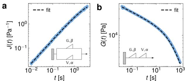
Fig. 2 Creep and stress relaxation data classified and fitted with pyRheo. (a) Creep compliance  $J(t)$  of a perihepatic abscess sample. The curve is fitted using the auto function in pyRheo, which classifies the data as a FractionalKelvinVoigt. (b) Relaxation modulus  $G(t)$  of a fish muscle classified and fitted with FractionalMaxwell. The raw data of the perihepatic abscess was reproduced from Shih *et al.*<sup>30</sup> and the data of the fish muscle from Song *et al.*<sup>2</sup>
