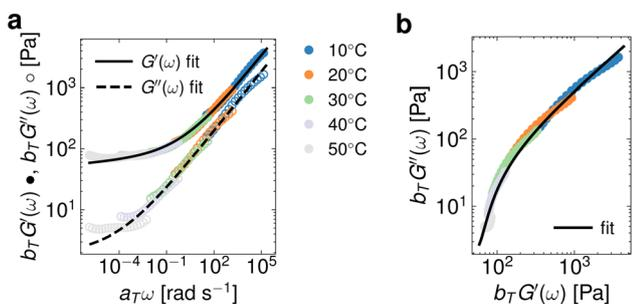
Fig. 3 Master curves for the linear viscoelastic behavior of an interpenetrating-network hydrogel made of cellulose nanofibers and methylcellulose. (a) Storage modulus  $G'(\omega)$  and loss modulus  $G''(\omega)$  master curves ( $T_{ref} = 30^\circ\text{C}$ ) constructed using the time-temperature superposition (TTS) and fitted with FractionalKelvinVoigt, constituted by two SpringPot models connected in parallel. (b) Cole-Cole representation of the master curve.
