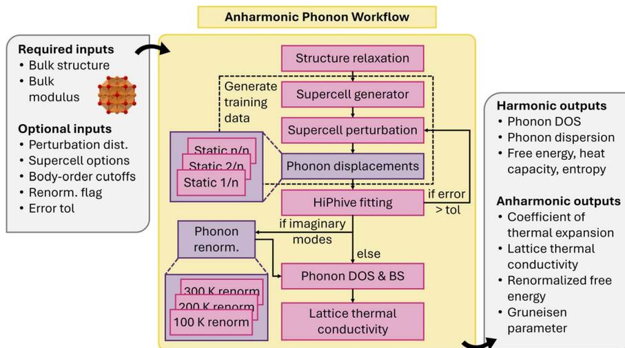
Fig. 13 Schematic of anharmonic phonon workflow.
