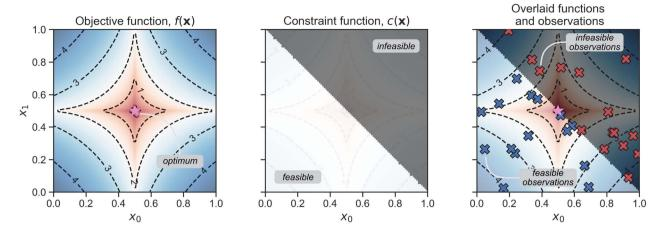
Fig. 1 Concept figure of an optimization problem with unknown constraints. The left-most subplot shows the contour plot of the objective function, f(x), with the global optimum marked with a pink star. The center subplot shows the binary constraint function, c(x). The right-most subplot shows the functions f(x) and c(x) overlaid on the same plot, with feasible (infeasible) measurement instances marked with blue (red) crosses.
