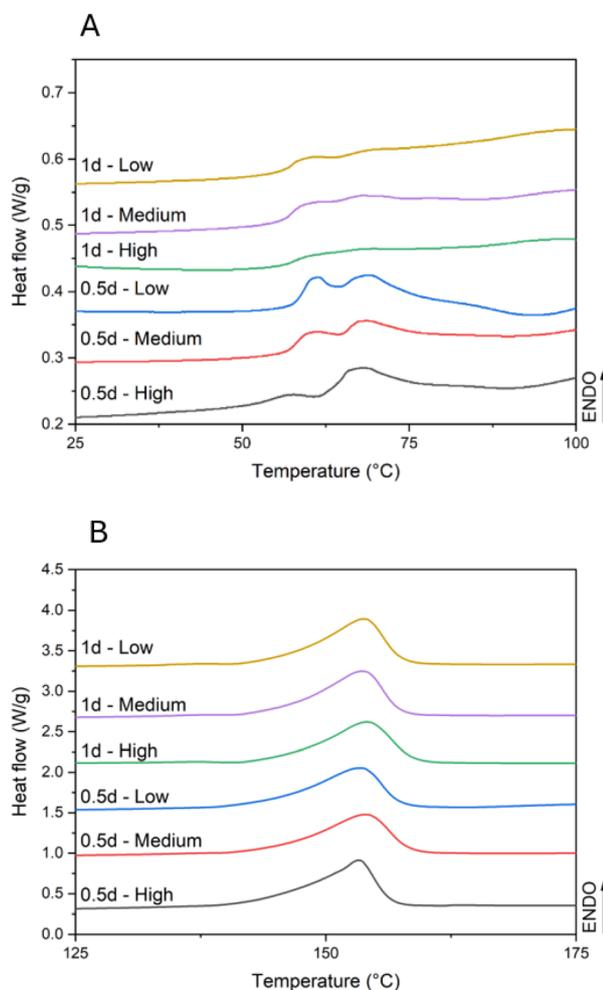
**Fig. 11** DSC thermograms (first heating curve) of injection-moulded PLA samples hydrolytically degraded in water at 60 °C for 0.5 day (0.5 d) and 1 day (1 d). Samples are categorized by impact strength level (high – highest value obtained, medium – medium value, low – lowest value obtained). (A) Glass transition temperature region (B) melting temperature region.
