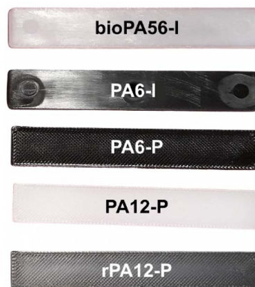
Fig. 4 Polyamide specimens used in water absorption experiment.
