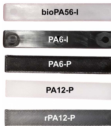
Fig. 4 Polyamide specimens used in water absorption experiment.
