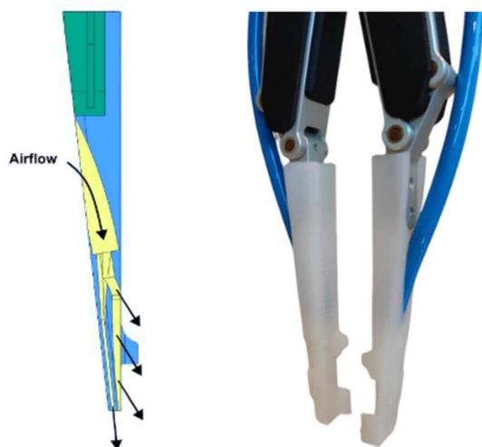
Fig. 2 End effector for UR10e robot arm with channeling for compressed air. On the right, schematic view of the gripper (blue) with the air circulation channels (yellow) and the robot mounting (green). On the left, 3D printed grippers mounted on the robot connected to 8 mm OD pneumatic tubing.
