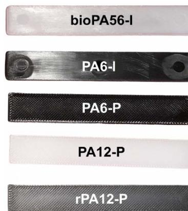
Fig. 4 Polyamide specimens used in water absorption experiment.
