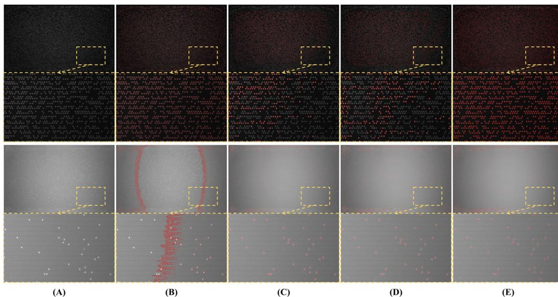
Fig. 5 Detection results of four different methods. (A) Raw. (B) Traditional thresholding algorithm, where red enclosed shapes (connected domains) represent positive detection results. (C) YOLOv5s-based direct prediction. (D) Improved YOLOv5s-based direct prediction. (E) Improved YOLOv5s-based partitioned fusion prediction. In (C–E), positive detections are marked with small red dots.
