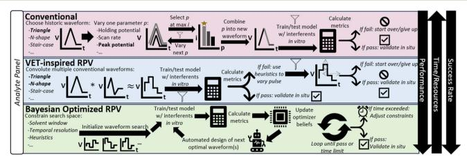
Fig. 1 Approaches to voltammetry waveform design. Funnels denote likely bottlenecks
