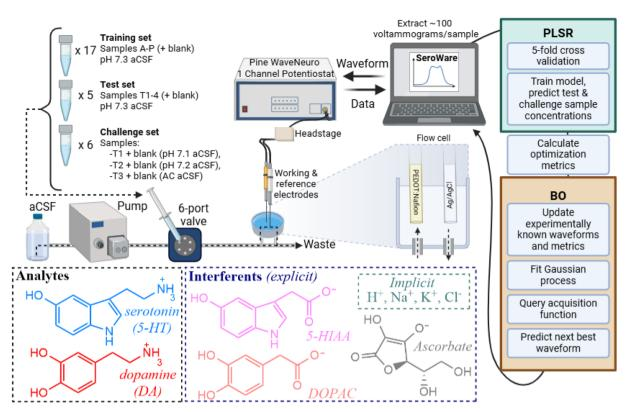
Fig. 7 Workflow for parallel Bayesian optimization of voltammetric waveforms with intrinsic interferent selectivity.
