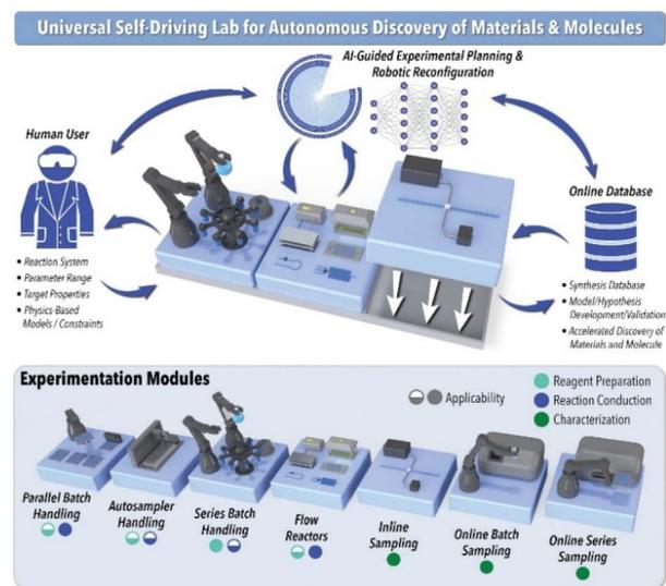
Fig. 3 Schematic Representation of a modular autonomous experimentation framework for a universal SDL. The generated experimental data can be utilized in decision-making algorithms and can be simultaneously stored in a centralized communal database. The human operator sets the operational constraints and defines the desired target properties or objectives for the system. Reproduced with permission. Copyright 2021, Elsevier.<sup>2</sup>
