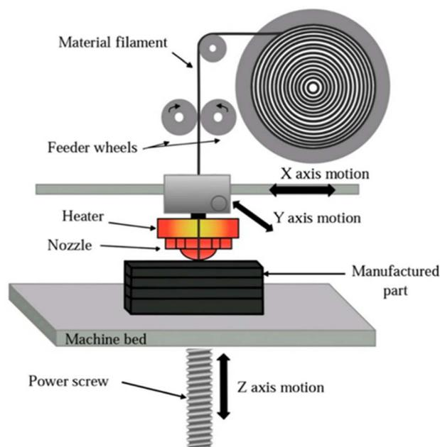
Fig. 8 A schematic representation of a Fused Deposition Modeling (FDM) 3D printing process. Reproduced with permission. Copyright 2023, Nature group.<sup>73</sup>
