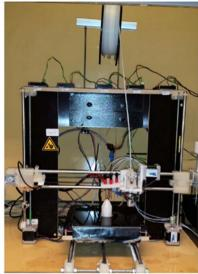
Fig. 18 Photographic view of a Prusa i3 RepRap printer modified into a robotic platform set-up with a 3D-printed reaction for the automated synthesis of ibuprofen Reproduced with permission. Copyright 2016, Beilstein Journal of Organic Chemistry. 157
