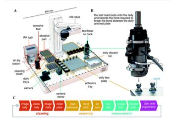
Fig. 7 (A) Schematic of a self-driving laboratory operating on a N9 adhesive material testing. (B) A close-up view of the hydraulic strength testing tool utilized by the robot to measure bond strength. (C) Flow chart of the workflow sequence of the system. Reproduced with permission. Copyright 2022, Royal Society of Chemistry. 16
