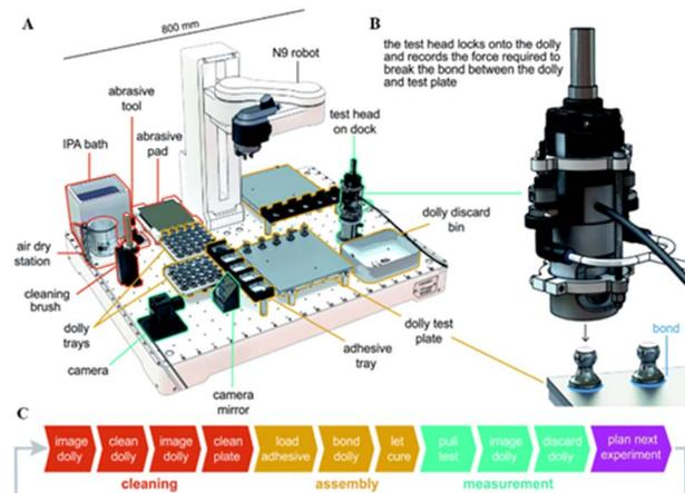
**Fig. 7** (A) Schematic of a self-driving laboratory operating on a N9 adhesive material testing. (B) A close-up view of the hydraulic strength testing tool utilized by the robot to measure bond strength. (C) Flow chart of the workflow sequence of the system. Reproduced with permission. Copyright 2022, Royal Society of Chemistry.<sup>16</sup>
