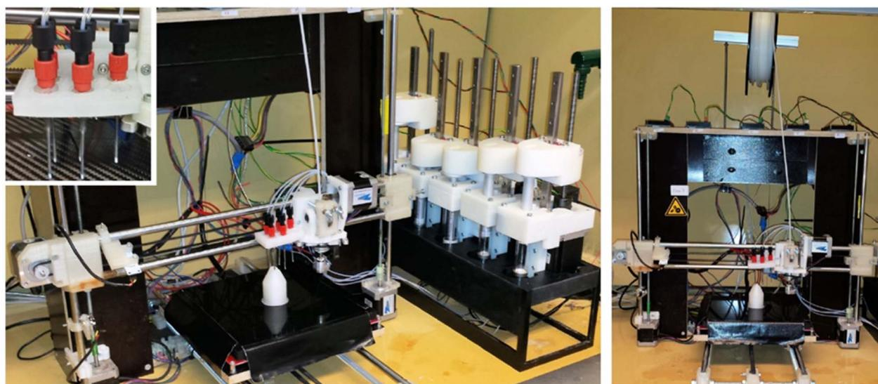
Fig. 18 Photographic view of a Prusa i3 RepRap printer modified into a robotic platform set-up with a 3D-printed reaction for the automated synthesis of ibuprofen. Reproduced with permission. Copyright 2016, *Beilstein Journal of Organic Chemistry*.<sup>157</sup>
