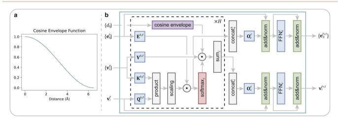
Fig. 2 The improved graph transformer used in DeepRLI. (a) The curve of the cosine envelope function. (b) Block diagram of the graph transformer with a cosine envelope.
