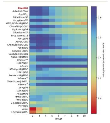
Fig. 5 A heatmap displaying the binding funnel landscapes of scoring functions. The ticks on the x-axis refer to the ranges of RMSDs (for example, 0–2Å, 0–3Å, etc.), and the corresponding blocks indicate the Spearman correlation coefficient between the RMSD values and the binding scores calculated using scoring functions for all ligand poses within these ranges.
