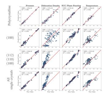
Fig. 8 Parity plots comparing the microstructural state descriptor regression accuracy for the state descriptors from the nanocrystalline shock-loading simulation for (top row) a model trained with dataset 11, (top middle) a model trained with dataset 4, (bottom middle) a model trained with dataset 8, and (bottom) a model trained with dataset 6. Values shown in parity plots are normalized based on the maximum and minimum values from their respective model training datasets.
