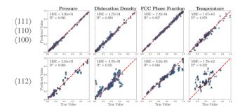
Fig. 7 Top row: validation set parity plots for a model trained with  $\langle111\rangle,~\langle110\rangle,~$  and  $\langle100\rangle$  orientations. Bottom row: parity plots for dataset 5 ( $\langle112\rangle$  orientation) created using a model trained with the orientations from the top row.
