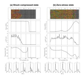
Fig. 3 Single crystal Cu shock loaded along  $\langle 111 \rangle$  in the (a) shock-compressed state and (b) zero-stress state, with the microstructure, Z stress, dislocation density, temperature, and fitted diffraction patterns of each bin shown. The five bins (I-V) taken along the Z direction are shown by dashed lines. The microstructure is colored by structure, where gray atoms correspond to FCC atoms, red to disordered atoms, and green for stacking faults.
