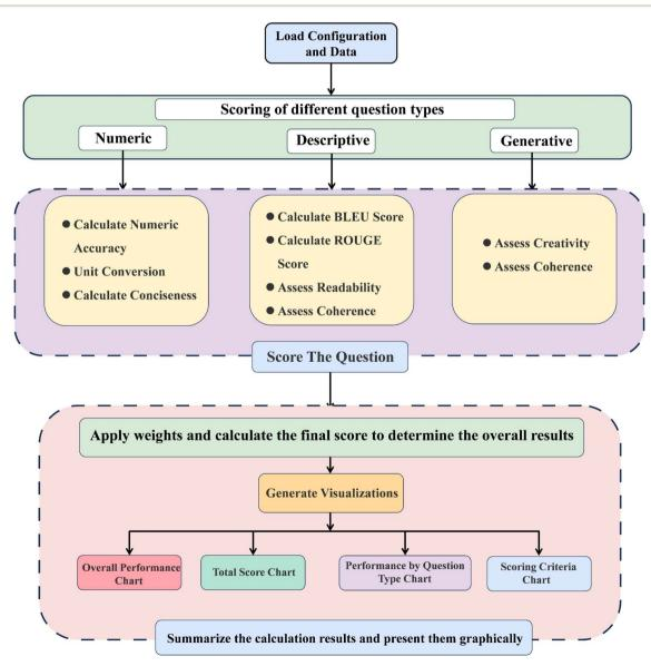
Fig. 8 Automatic grading program process.
