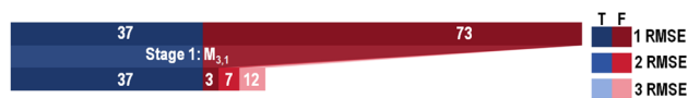
Fig. 6 A one-stage screening workflow for materials with a triplet excitation energy in the infrared, below 1.6 eV, based on the M_{3,1} model. The number of true positives (shades of blue) and the number of false positives (shades of red/pink) that pass the screening is shown when the thresholds are set to one, two, and three times the training set RMSE of the model.
