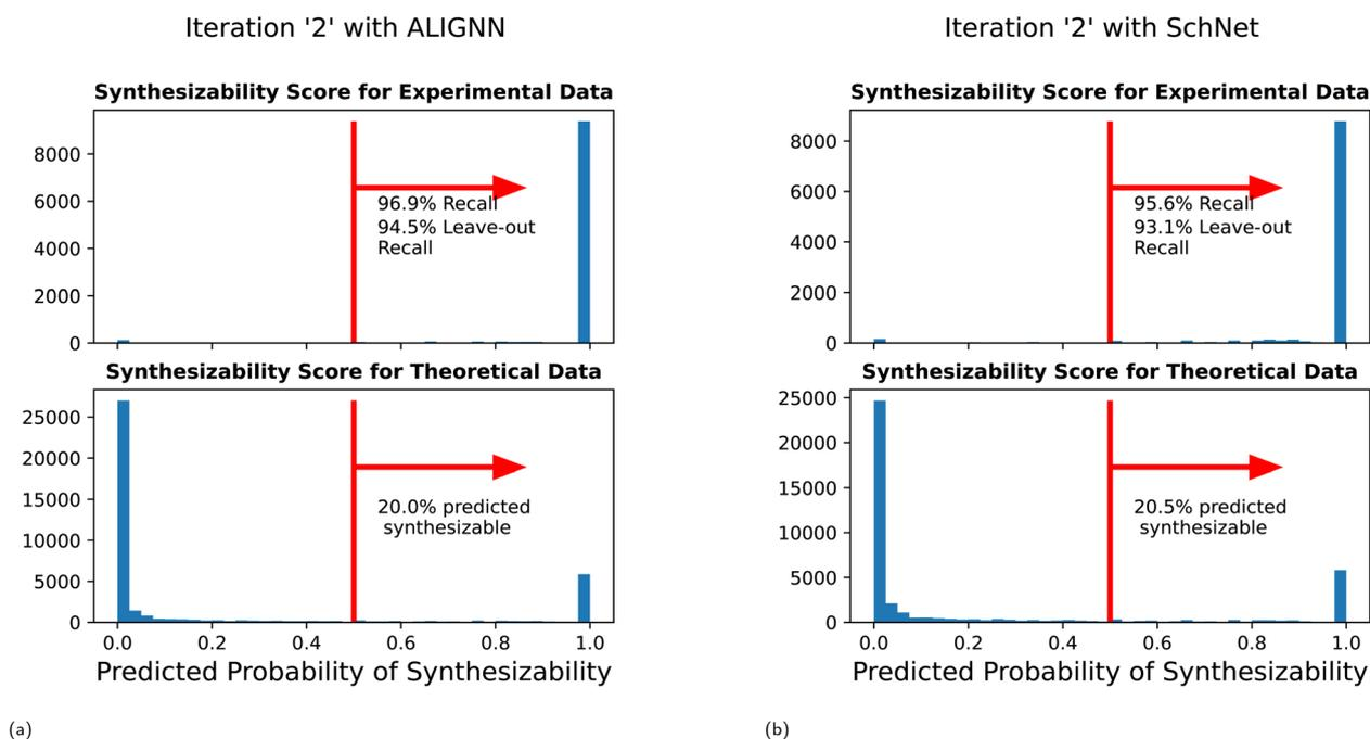
**Fig. 4** Synthesizability score distribution for Iteration '2' for the (a) ALIGNN0 series and (b) SchNet0 series. We observe a bimodal distribution emerging in the unlabeled data, while the experimental data maintains a single peak. The bimodality results from the co-training mechanism, where positively predicted materials are integrated into the positive set of the training data.
