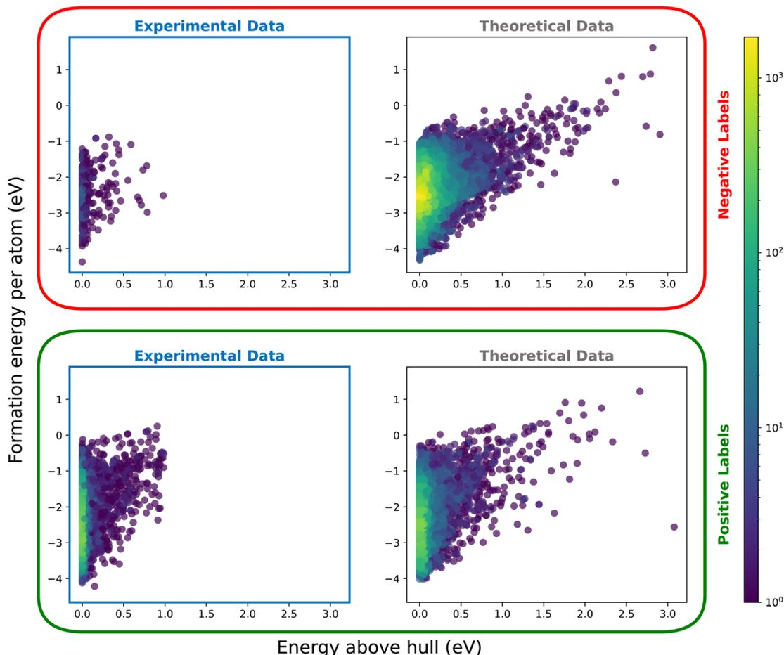
Fig. 7 Distribution of formation energy versus energy above hull for experimental data (left) and theoretical data (right), separated by predicted labels. The figure illustrates the expected clustering of positively labeled data around lower values of energy above hull while no distinct density peaks are observed with respect to formation energy.
