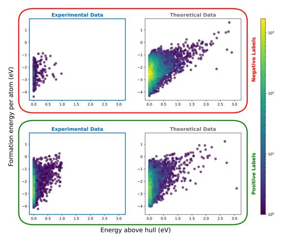
Fig. 7 Distribution of formation energy *versus* energy above hull for experimental data (left) and theoretical data (right), separated by predicted labels. The figure illustrates the expected clustering of positively labeled data around lower values of energy above hull while no distinct density peaks are observed with respect to formation energy.
