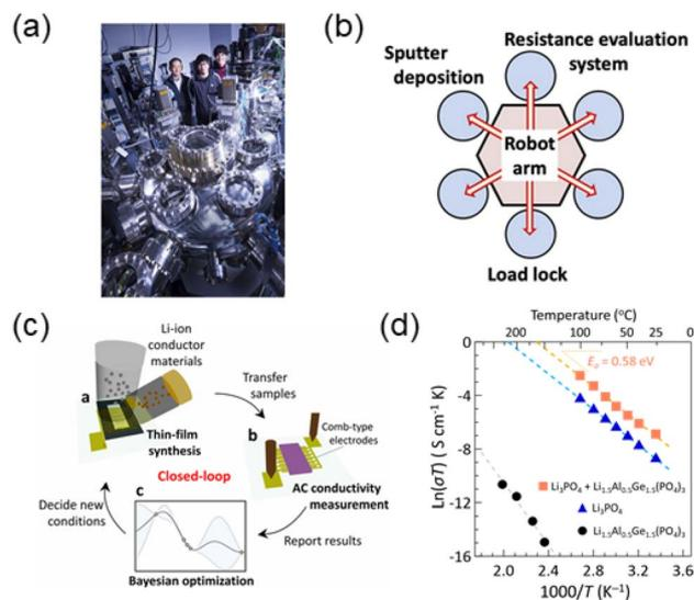
Fig. 2 (a) Photograph and (b) schematic of autonomous experimental system for exploration of inorganic thin-film materials. Copyright 2020 Shimizu *et al.*<sup>7</sup> and reprinted with permission under CC BY 4.0. (c) Autonomous experimental cycle for exploration of ionic conductors. (d) Ionic transport properties of fabricated amorphous ionic conductors thin films. Reprinted with permission from Kobayashi *et al.*<sup>8</sup> Copyright 2023 American Chemical Society.
