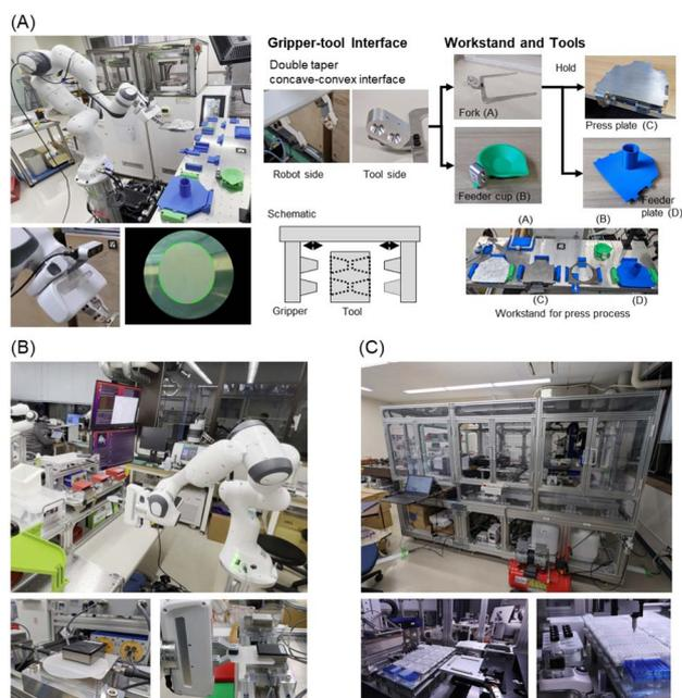
Fig. 5 (A) Press process automation system for polymer materials development, adapted from Asano *et al.*<sup>28</sup> (B) Dielectric property measurement system. Reprinted with permission from Asano *et al.*<sup>29</sup> Copyright 2024, IEEE. (C) Automation system for heat transfer materials development.
