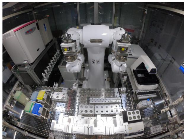
Fig. 8 The LabDroid Maholo including peripheral equipment. Reprinted from Kanda *et al.*<sup>38</sup> under CC BY 4.0.
