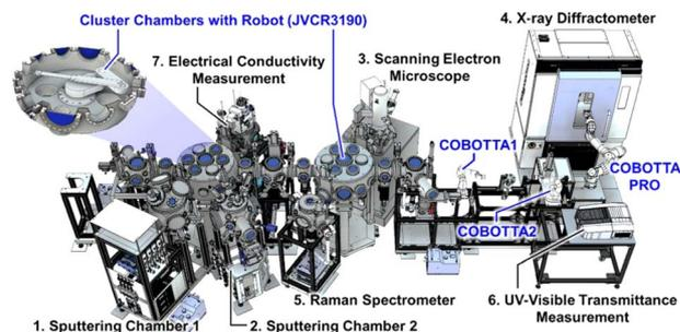
Fig. 12 Schematic of the digital laboratory (dLab) for thin film materials.<sup>131</sup>
