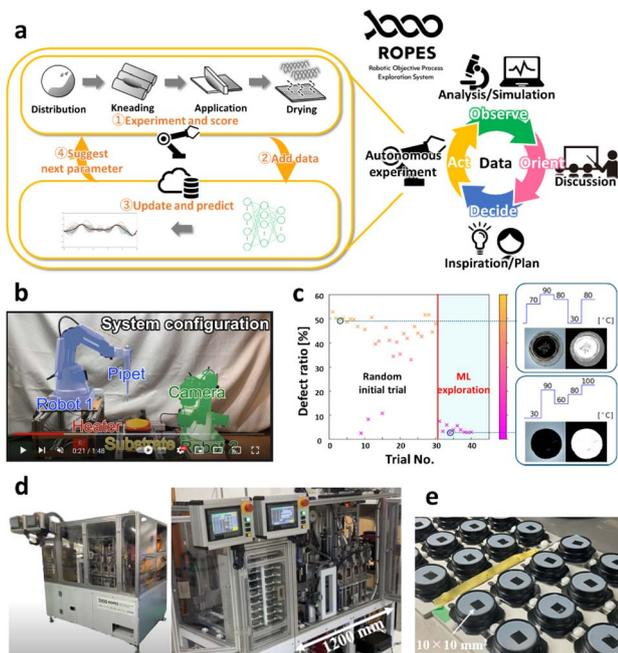
Fig. 7 ROPES of powder-film-formation-process, (a) schematic of an autonomous system, (b) experimental setup with two robot hands,<sup>36</sup> (c) results of exploration of drying process parameters minimizing defect ratio,<sup>34</sup> (d) a scalable autonomous system, (e) high-throughput prototyped fuel cell catalyst layer samples. A video about ROPES is available online.<sup>35</sup>
