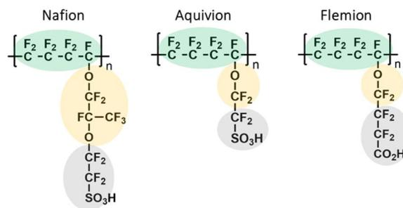
Fig. 1 Chemical structures and coarse-graining method for Nafion<sup>TM</sup>, Aquivion<sup>®</sup>, and Flemion<sup>TM</sup>. The green (segment A) represents the perfluorinated backbone, the yellow (segment B) corresponds to the branching structures, and the gray (segment C) denotes the sulfonic acid (–SO<sub>3</sub>H) or carboxylic acid (–CO<sub>2</sub>H) functional groups, which play a key role in phase separation.
