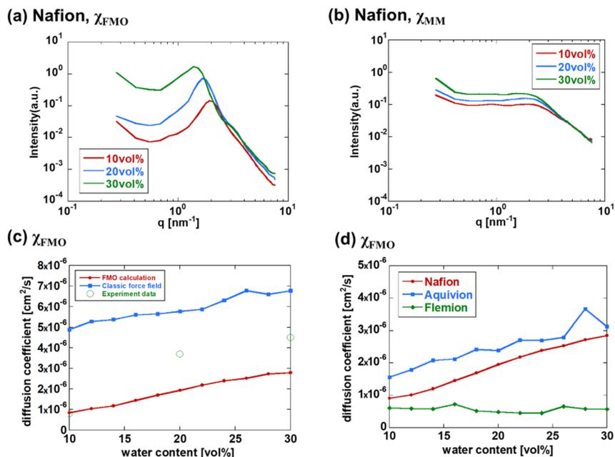
Fig. 4 Water-content-dependent small-angle scattering patterns for Nafion™ obtained from dissipative particle dynamics (DPD) simulations using (a)  $\chi_{FMO}$  and (b)  $\chi_{MM}$ . (c) Water diffusion coefficient obtained from DPD simulations using  $\chi_{FMO}$  and  $\chi_{MM}$ . Experimental values reported in ref. 54 are also plotted. (d) Water diffusion coefficients of Nafion™ (red), Aquivion® (blue), and Flemion™ (green). Values are averages from five DPD simulations.
