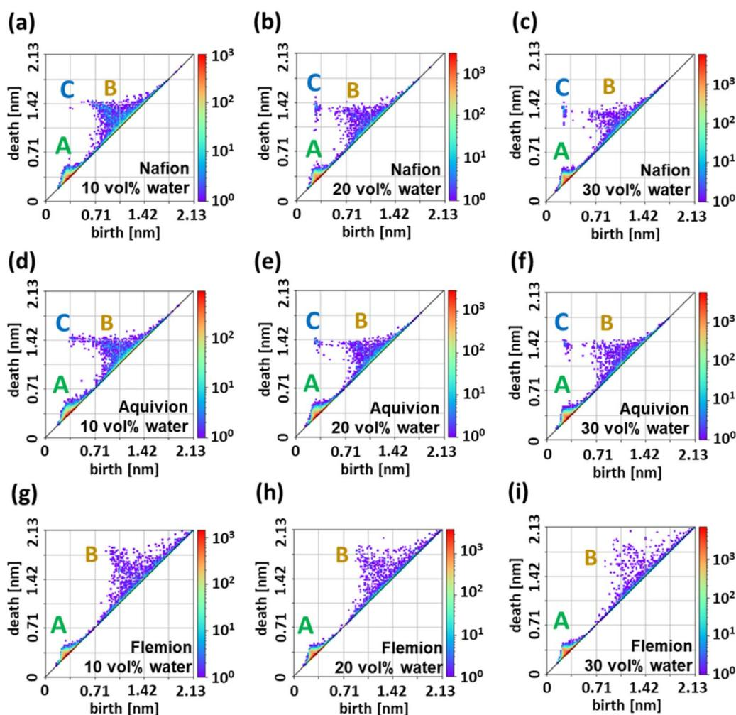
Fig. 5 Persistence diagrams (PDs) of water particles in (a, d and g) 10, (b, e and h) 20, and (c, f and i) 30 vol% hydrated (a–c) Nafion™, (d–f) Aquivion®, and (g–i) Flemion™. The color bar represents the number of topological features in each region of the diagram, with warmer colors (red) indicating higher densities and cooler colors (blue/green) indicating lower densities.
