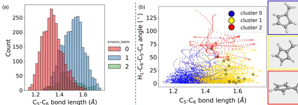
Fig. 12 (a) Histogram showing the distribution of  $C_5-C_6$  bond distances (in Å) categorized by  $K$ -means cluster labels. Each color represents a different cluster. (b) Scatter plot of the  $H_1-C_6-C_5-C_4$  dihedral angle versus the  $C_5-C_6$  bond length, with points colored according to their corresponding cluster. Representative geometries for each cluster are displayed alongside the plot.
