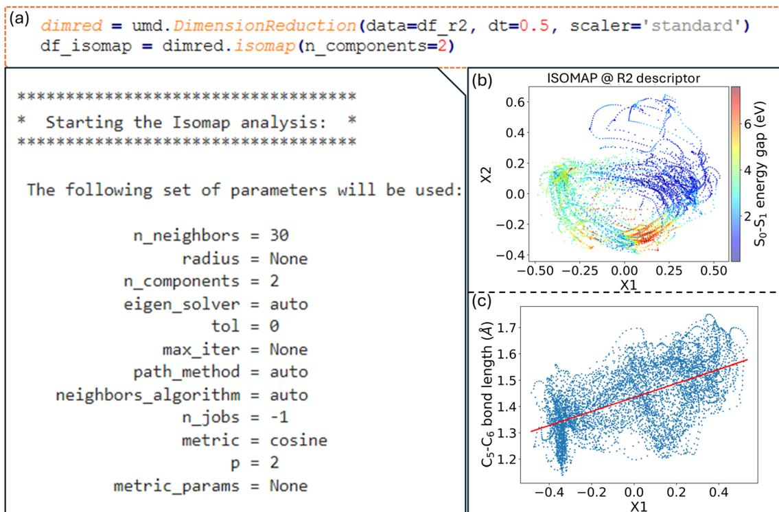
Fig. 8 (a) Dimensionality reduction using ISOMAP in ULAMDyn, with the parameters for the ISOMAP analysis; (b) the 2D ISOMAP embedding of the R2 descriptor, with the  $S_0$ - $S_1$  energy gap color-coded; (c) the relationship between the first ISOMAP component and the  $C_5$ - $C_6$  bond distance.
