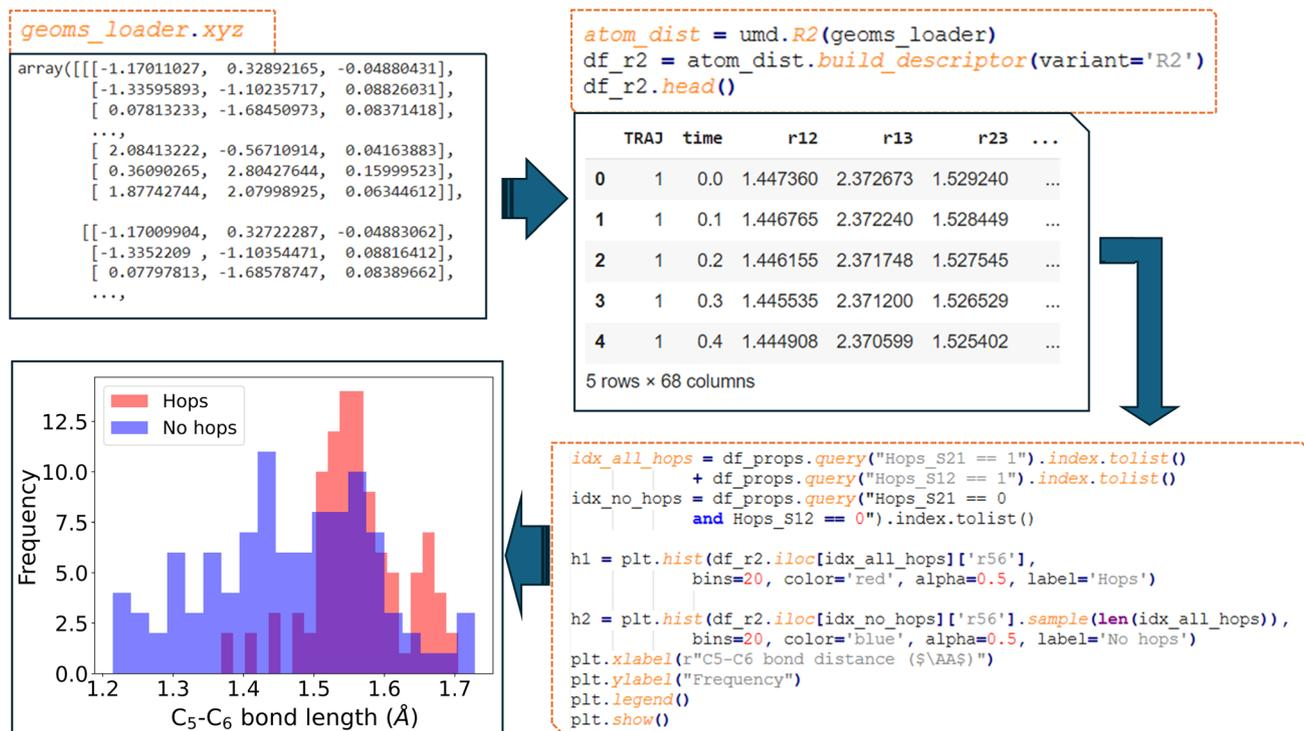
Fig. 6 Workflow demonstrating the use of ULaMDyn to generate descriptors and visualize results. The left panel shows the raw coordinates loaded from NAMD simulations. These coordinates are used to build an R2 descriptor ( $df\_r2$ ), as seen in the top-right panel. The bottom-right panel presents the code to create a histogram comparing C<sub>5</sub>-C<sub>6</sub> bond distances for geometries with and without hopping events, with the resulting histogram displayed in the bottom-left panel.
