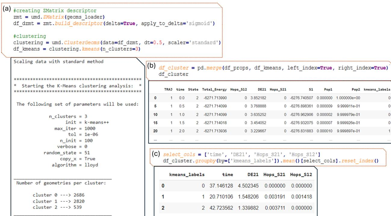
Fig. 10 (a) The Z-matrix descriptor is created for geometries, followed by clustering using *K*-means (with 3 clusters). The parameters for *K*-means are detailed, showing the number of geometries in each cluster; (b) the clustered data is then merged with properties data (*df\_props*); (c) the average values of selected properties (DE21, Hops\_S21, Hops\_S12) are computed for each cluster.
