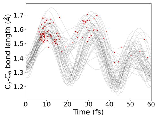
Fig. 7 Stretching of C<sub>5</sub>-C<sub>6</sub> bond length of fulvene for 50 trajectories. Points in red indicate the hopping events, which mainly occur at the maximum bond length.
