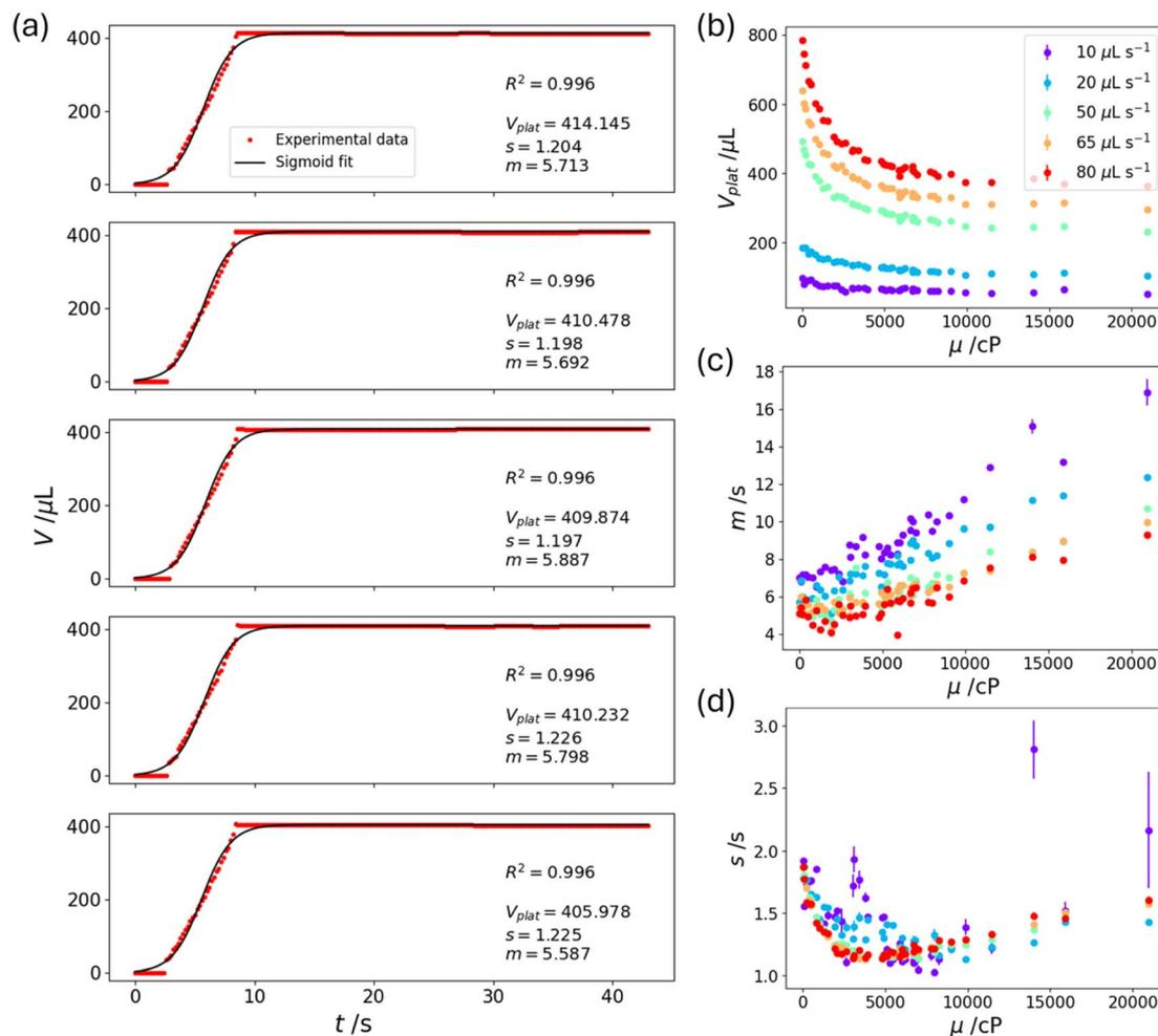
**Fig. 3** Sigmoid fits to the dispense curves. (a) Five replicates of the measurement protocol for a Newtonian standard with viscosity of 6033 cP at a set dispense flow rate of  $80 \mu\text{L s}^{-1}$ . The black lines are fits of eqn (1) to the red experimental data points. The fit parameters to eqn (1) for all measured viscosities and set dispense flow rates are plotted: (b)  $V_{\text{plat}}$ , (c)  $m$  and (d)  $s$ .
