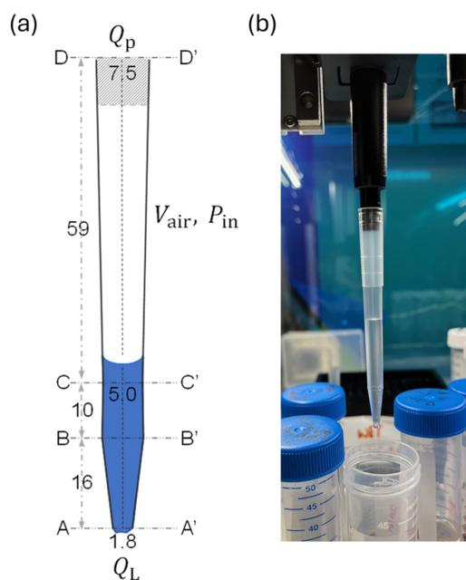
Fig. 5 Experimental setup (a) schematic of pipette tip and (b) photograph of Thermo Scientific 1000  $\mu\text{L}$  wide bore pipette after the aspiration stage. Diameter of the duct at locations AA', BB'/CC' and DD' and distances AB, BC and CD indicated, all dimensions in mm.
