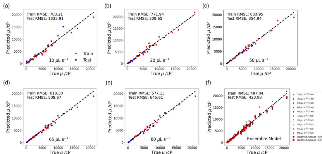
Fig. 4 Support vector regression model trained on data at different set dispense flow rates: (a)  $10 \mu\text{L s}^{-1}$ , (b)  $20 \mu\text{L s}^{-1}$ , (c)  $50 \mu\text{L s}^{-1}$ , (d)  $65 \mu\text{L s}^{-1}$  and (e)  $80 \mu\text{L s}^{-1}$ . Predictions from the model trained on datasets collected at each set dispense flow rate are weighted by the train RMSE value and averaged to produce an ensemble model.
