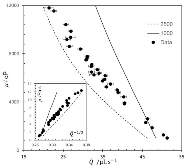
Fig. 7 Comparison of predicted effect of viscosity on average flow rate for Newtonian viscosity standards reported by Soh *et al.* (2023) for tests with dispense period of 5 s and  $Q_p = 50 \mu\text{L s}^{-1}$ . Error bars indicated 95% confidence interval from 9 repeats. Loci show predictions of simplified model, eqn (14), with parameters  $P_0 = 101325 \text{ Pa}$ ,  $V_0$  values indicated. Inset shows the data in the linearized form reported by Soh *et al.*
