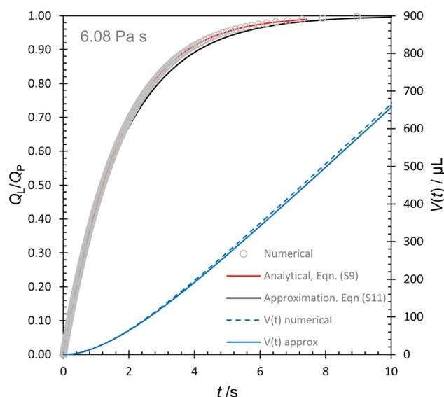
Fig. 6 Predicted evolution of scaled flow rate and volume dispensed from the pipette tip in Fig. 5 for a 6.08 Pa s Newtonian liquid with  $Q_p = 80 \mu\text{L s}^{-1}$ ,  $P_0 = 101325 \text{ Pa}$  and  $V_0 = 2000 \mu\text{L}$ .
