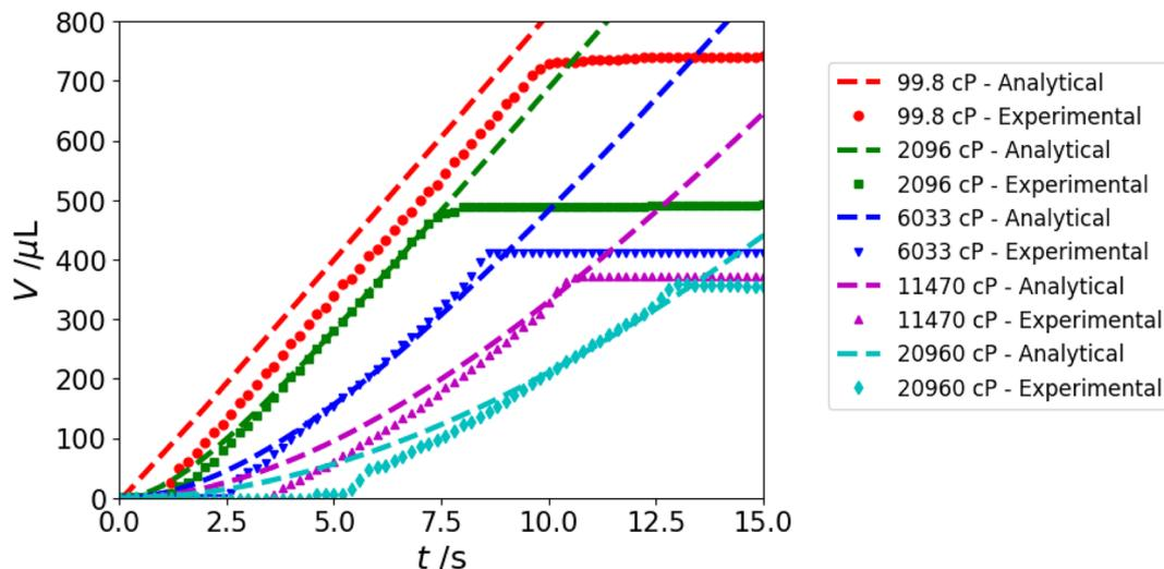
Fig. 9 Comparison between analytical model and experimental data for Newtonian fluids with different viscosities at a set dispense flow rate of  $80 \mu\text{L s}^{-1}$ . Points – experimental data. Dotted lines – model predictions, with  $P_0 = 95 \text{ kPa}$  and  $V_0 = 8000 \mu\text{L}$ .
