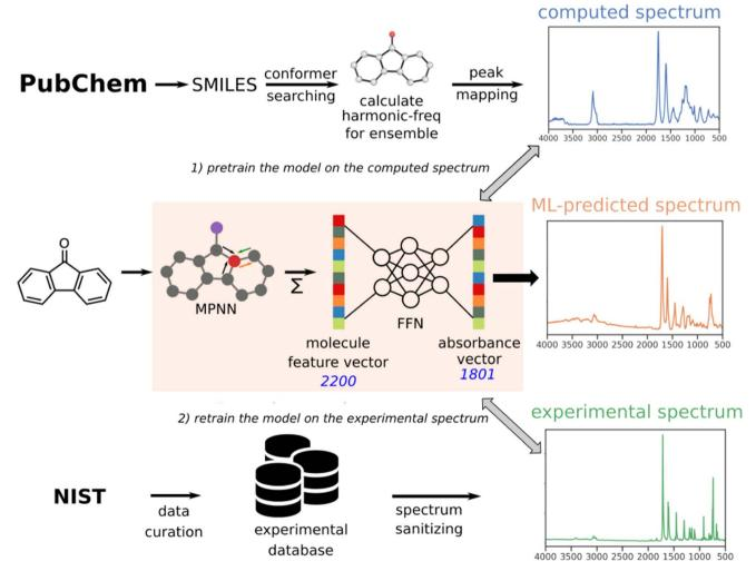
Fig. 21 Workflow of the chemprop-IR model, which was pretrained with computed spectra on ~85k PubChem molecules and retrained with ~57k experimental spectra. Reprinted with permission from the American Chemical Society Copyright (2021). 184
