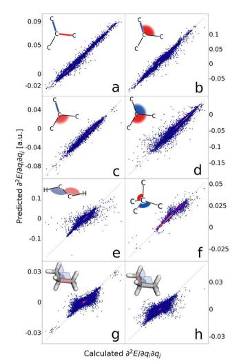
Fig. 17 Parity plots comparing predicted and calculated non-diagonal terms of the Hessian matrix. (a) Consecutive bond-bond. (b) included bond-angle, (c) adjacent bond-angle, (d) adjacent angle-angle, (e) consecutive angle-angle, (f) opposite angle-angle, (g) external bonddihedral, and (h) internal bond-dihedral. Reprinted under CC BY 4.0 license from ref 176
