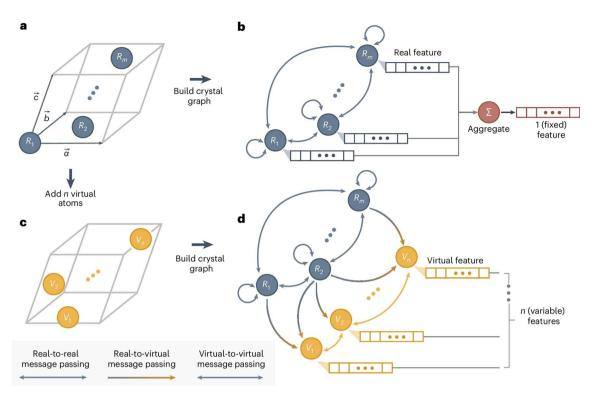
Fig. 7 Design of virtual node GNN. (a) A crystal structure, which is converted into (b) a crystal graph in a GNN with real nodes. (c) By adding virtual nodes to the crystal structures, the (d) virtual node graph can be used to represent both atoms and collective excitations, where the unidirectional information passing from real nodes to virtual nodes ensures the training quality. Reprinted with permission from Springer Nature Copyright (2024).93
