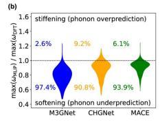
Fig. 12 Comparison of three UIPs and DFT for phonon calculations. (a) Phonon dispersion and DOS of CsF, calculated using DFT and various UIPs. (b) Violin plots showing the distribution of ratios between maximum frequencies calculated by UIPs and DFT, for 229 crystals. Systematic and significant softening is observed in the phonon frequencies calculated by the UIPs. Reprinted under CC BY 4.0 license from ref. 141.
