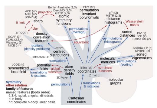
Fig. 5 Phylogenetic tree of representations of atomic structures. Arrows indicate the relationship (blue: symmetry; red: other relation) between different hierarchies of structural features. The atomic density fields and the internal coordinates of an atom are two approaches for molecular and crystal structure representation. Reprinted under CC BY 4.0 license from ref. 70.
