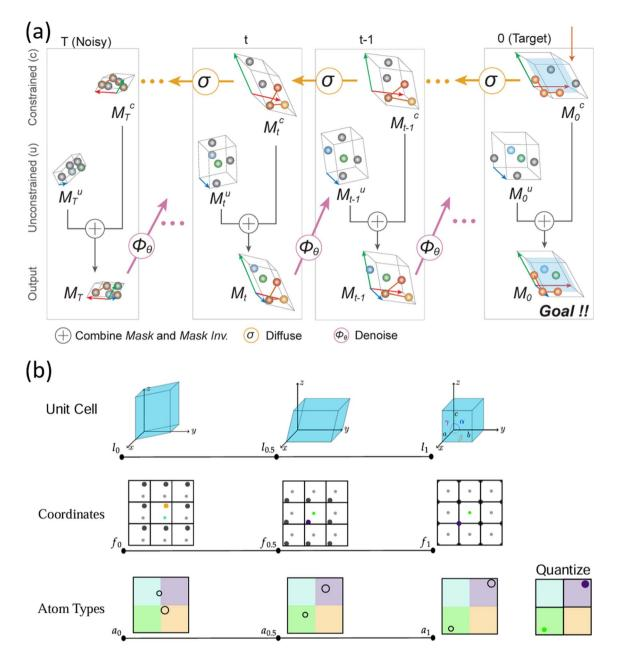
Fig. 24 Examples of generative models for discovering new materials. (a) SCIGEN. Reprinted under CC BY 4.0 license from ref. 212. (b) FlowMM. Reprinted under CC BY 4.0 license from ref. 213.
