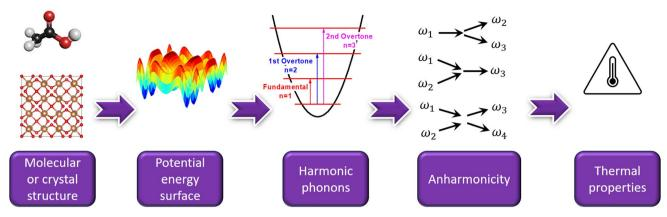
Fig. 1 A typical workflow to compute a material's vibrational and thermal properties from its molecular or crystal structure.
