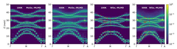
Fig. 13 Phonon spectral energy density calculated by Gupta et~al. for MoSe<sub>2</sub> and WSe<sub>2</sub> using molecular dynamics and MLIPs. The effects of anharmonicity can be clearly seen in the 500 K spectra as the broadening of the lines and the diffusive intensities. Reprinted with permission from Royal Society of Chemistry Copyright (2023).
