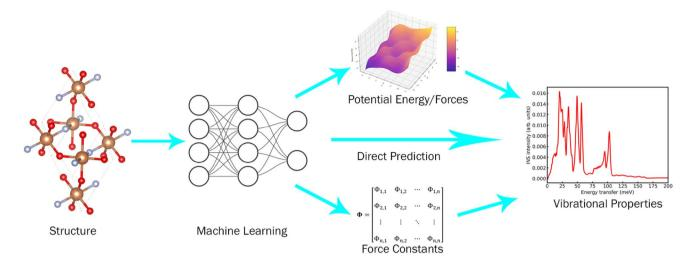
Various routes towards data-driven prediction or calculation of the vibrational dynamics and spectra
