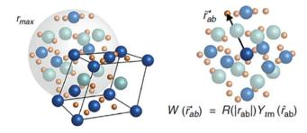
Fig. 6 Sketch of a symmetry-aware representation of atomic structure using e3nn. (Top) An atomic structure is converted into a crystal graph with nodes and edges, and when structural information passes within a cutoff radius  $r_{\text{max}}$  for a given atom, the angular information and radial information between two atoms are encoded in spherical harmonics  $Y_{lm}(r_{ab})$  and a radial neural network  $R(|r_{ab}|)$ , respectively. Reprinted under CC BY 4.0 license from ref. 90.
