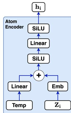
Fig. 7 Schematic of the atom encoder used in CartNet. The encoder processes each atomic number ( $Z_i$ ) using an embedding layer and its temperature using a linear layer. The resulting encoded features are summed and passed through a SiLU activation function, followed by an additional linear layer and another SiLU. The final vector  $h_i$  serves as the initial node features for the CartLayer.
