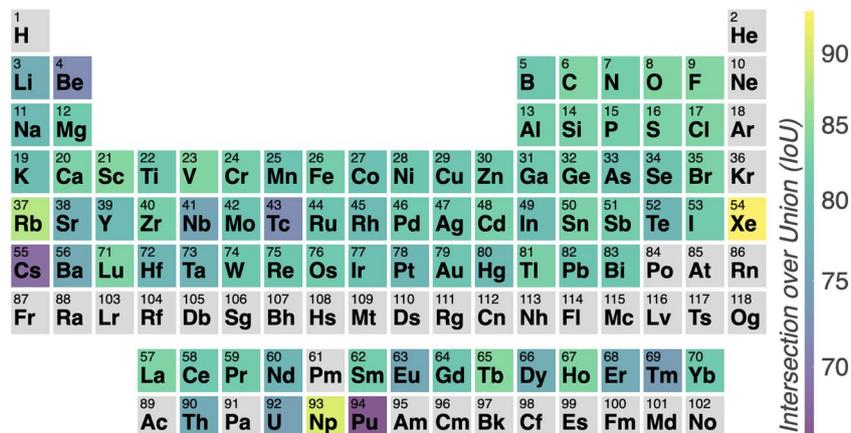
Fig. 15 Heatmap illustrating the IoU metric per element for the CartNet's predictions in the test split from the ADP dataset. Lighter colours represent higher IoU, while darker colours indicate lower IoU.
