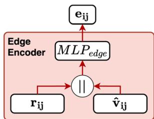
Fig. 8 Schematic of the edge encoder used in CartNet. The  $\mathbf{e}_{ij}$  and the  $\hat{\mathbf{v}}_{ij}$  are concatenated and then processed by a  $MLP_{edge}$  to generate the initial edge features utilized by the CartLayer.
