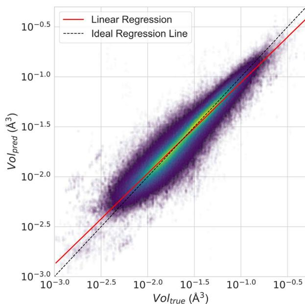
**Fig. 12** Scatter plot of true versus predicted ADP volumes for the test split of the ADP dataset using CartNet. A linear regression fitted to the data yields  $y = 1.0013x + 0.0021$  with an  $R^2$  score of 0.91, indicating a correlation. The scale is logarithmic for both axes.
