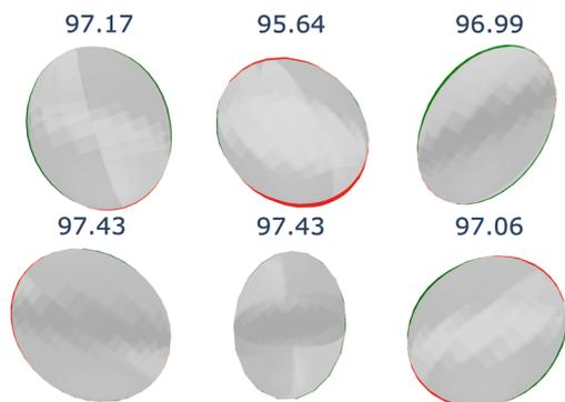
**Fig. 18** Visualization of rotational errors by comparing the rotated ADP predictions from the original crystal structures (green ellipsoids,  $RU_{\text{orig}}R^T$ ) with the ADP predictions from the rotated crystal structures (red ellipsoids,  $U_{\text{rot}}$ ). The overlapping regions are shaded in grey, representing the intersection between the two predictions. The IoU values are displayed above each pair of ellipsoids.
