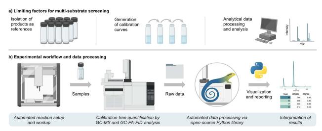
Fig. 1 (a) Challenges in HTE for multi-substrate screenings. (b) Experimental workflow comprising automated reaction setup and workup, GC-MS and GC-PA-FID analysis, and data processing via the open-source pyGecko library.
