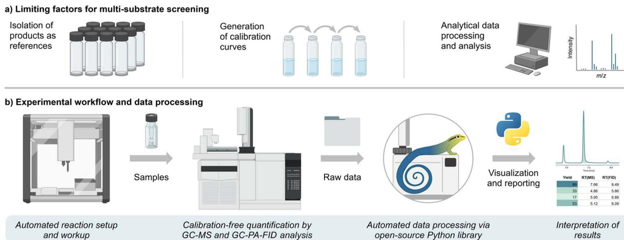
**Fig. 1** (a) Challenges in HTE for multi-substrate screenings. (b) Experimental workflow comprising automated reaction setup and workup, GC-MS and GC-PA-FID analysis, and data processing via the open-source pyGecko library.
