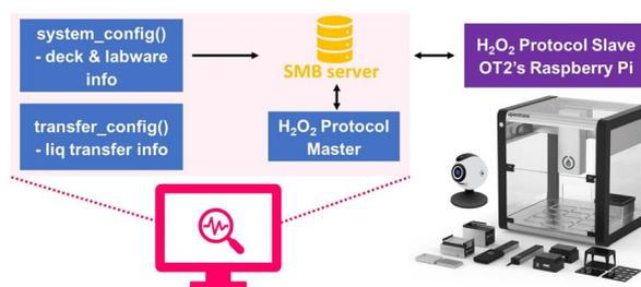
Fig. 4 The illustration of the interactive working system for HTE  $H_2O_2$  determination (SMB server – service message block, OT-2 image reprinted with permission from OpenTrons. Copyright OpenTrons).
