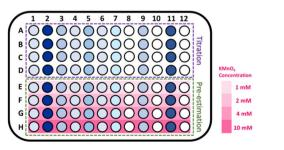
Fig. 2 Illustration of the experimental layout of a 96-well white plate. The shades of blue represent the different concentrations of  $H_2O_2$  sample. The green area was used for pre-estimation, while the purple area was used for titration.
