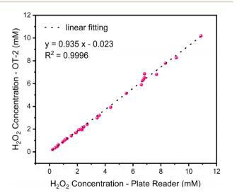
Fig. 5 Sensitivity test  $(x - H_2O_2)$  concentration determined by the plate reader,  $y - H_2O_2$  concentration determined by the liquid robot Opentrons (OT-2)).
