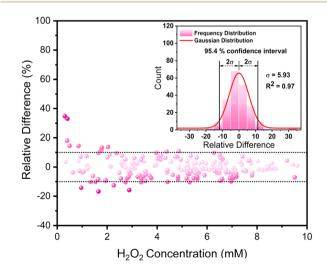
Fig. 6 The relationship between relative difference and  $H_2O_2$  concentration (the lighter the pink dot is, the closer the relative difference is zero). The inset plot is the frequency distribution of relative difference (bin range:  $\pm 30\%$ , bin width: 5%) and its corresponding Gaussian distribution ( $x_c = 0, y_0 = 2$ ) as shown in the red line.
