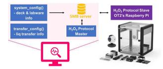
Fig. 4 The illustration of the interactive working system for HTE H<sub>2</sub>O<sub>2</sub> determination (SMB server - service message block, OT-2 image reprinted with permission from Opentrons. Copyright Opentrons).
