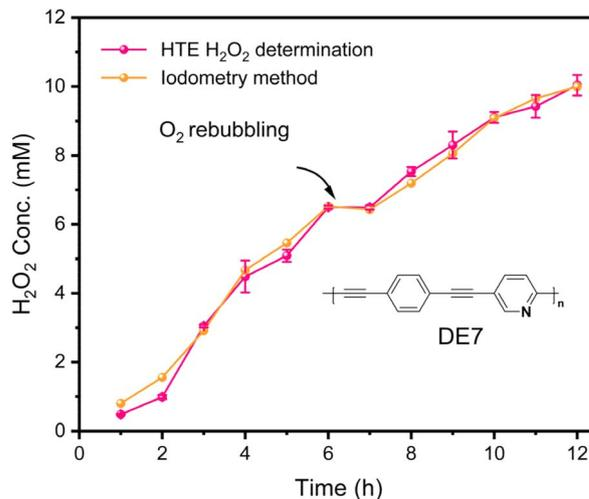
Fig. 7 The  $\text{H}_2\text{O}_2$  photoproduction over photocatalyst DE7. The error bar is the standard deviation of HTE  $\text{H}_2\text{O}_2$  determination, where each sample was measured four times in parallel.
