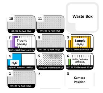
Fig. 1 The deck layout of OT-2 for HTE  $H_2O_2$  determination using an automated liquid-handing robot OT-2 (purple = potassium permanganate solution of known concentration, KMnO<sub>4</sub>; yellow =  $H_2O_2$  samples of unknown concentration; blue = pure water; green = 1 M sulfuric acid,  $H_2SO_4$ ). Deck number was placed in the upper left corner of each grid.
