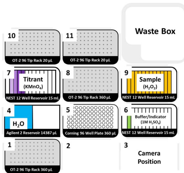
Fig. 1 The deck layout of OT-2 for HTE  $\text{H}_2\text{O}_2$  determination using an automated liquid-handling robot OT-2 (purple = potassium permanganate solution of known concentration,  $\text{KMnO}_4$ ; yellow =  $\text{H}_2\text{O}_2$  samples of unknown concentration; blue = pure water; green = 1 M sulfuric acid,  $\text{H}_2\text{SO}_4$ ). Deck number was placed in the upper left corner of each grid.
