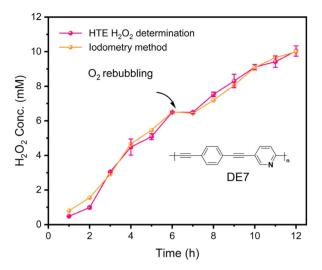
Fig. 7 The H<sub>2</sub>O<sub>2</sub> photoproduction over photocatalyst DE7. The error bar is the standard deviation of HTE H<sub>2</sub>O<sub>2</sub> determination, where each sample was measured four times in parallel.
