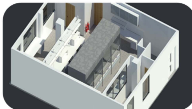
Fig. 4 (Top left, clockwise) Process of developing a digital twin model in VR, utilising existing floor plans to develop accurate CAD models with further optimisation in Revit and Unreal Engine.
