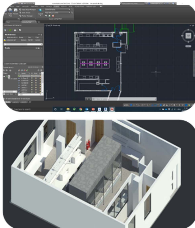
Fig. 4 (Top left, clockwise) Process of developing a digital twin model in VR, utilising existing floor plans to develop accurate CAD models with further optimisation in Revit and Unreal Engine.
