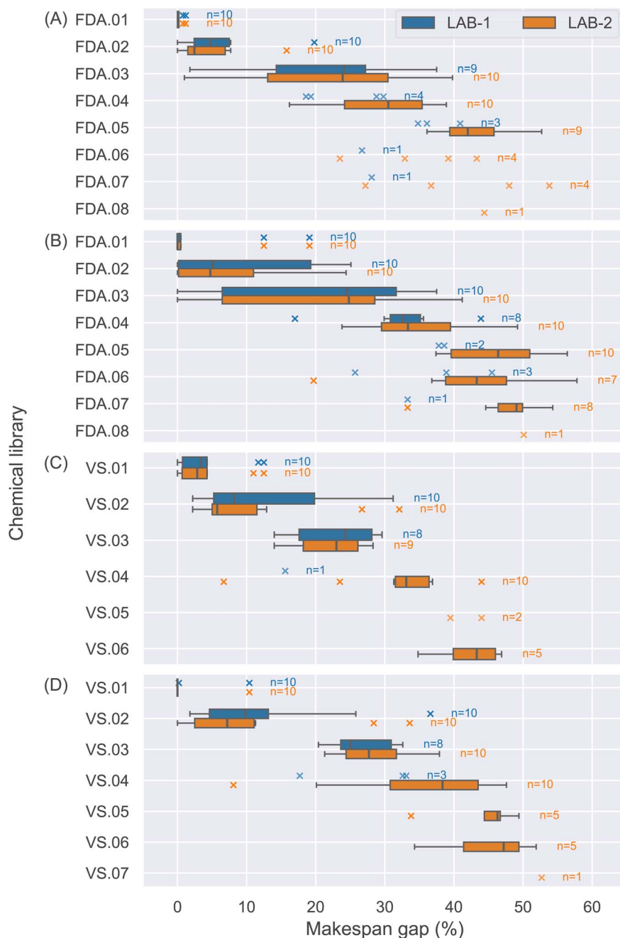
Fig. 4 Percentage makespan gaps between baseline and optimal MILP schedules. Two types of markers denote scheduling instances on LAB-1 and LAB-2, respectively. (A) FDA libraries without work shift constraints; (B) FDA libraries with work shift constraints; (C) VS libraries without work shift constraints; (D) VS libraries with work shift constraints. The percentage gap ranges from 0% to 57.8%, and tends to be higher for larger libraries. Percentage gaps were calculated based on the makespan values of baseline schedules.
