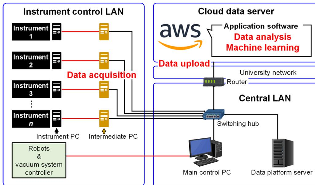
Fig. 2 Network configuration diagram of the system. The black lines indicate networks connected to the external network, whereas the red lines represent networks isolated and protected from external access. Each synthesis and measurement/analysis module is connected to the main control PC via intermediate PCs. The internal network links the system to a cloud-based data server.
