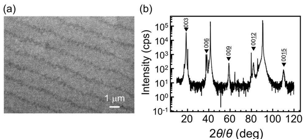
Fig. 5 (a) Scanning electron microscopy image of the  $\text{LiCoO}_2$  thin film. This image was taken at an accelerating voltage of 10.0 kV and a magnification of 10 000. It is possible to observe at a magnification of up to 100 000. The striped patterns observed in the SEM image are caused by surface structures on the  $\text{LiCoO}_2$  surface. (b) Raw data of the out-of-plane X-ray diffraction pattern of the  $\text{LiCoO}_2$  thin film.
