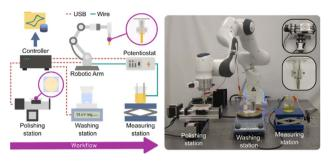
Fig. 1 Automated electrode polishing workflow. The robot moves the electrode between the polishing, washing and measuring stations to automatically activate the electrode by polishing and run cyclic voltammetry measurements using the potentiostat. The complete procedure is conducted without human intervention.
