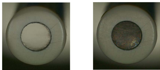
Fig. 3 Photo of the surface of a glassy carbon electrode before (left) and after (right) corrosion, which was taken during our preliminary experiment. The electrode was applied a 3.3 V potential for 600 seconds inside 0.5 M sodium sulphate solution. Note that a higher voltage (5 V) was used in the actual experiment to cause corrosion quickly and in a controlled manner.
