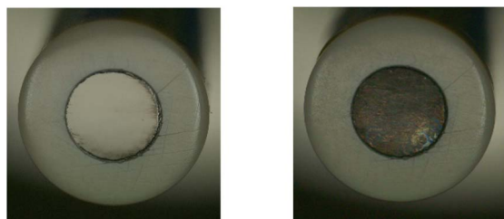
Fig. 3 Photo of the surface of a glassy carbon electrode before (left) and after (right) corrosion, which was taken during our preliminary experiment. The electrode was applied a 3.3 V potential for 600 seconds inside 0.5 M sodium sulphate solution. Note that a higher voltage (5 V) was used in the actual experiment to cause corrosion quickly and in a controlled manner.
