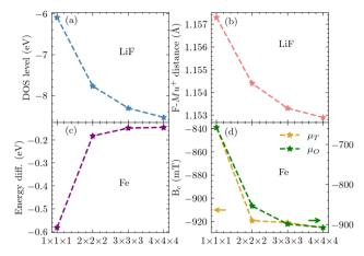
Fig. 4 Convergence of muon-related relaxed calculations vs. supercell size. LiF: (a) position of the Mu<sup>+</sup> DOS peak with respect to the Fermi energy, and (b) F–Mu<sup>+</sup> distance. Fe: (c) total energy difference between  $\mu_T$  and  $\mu_O$ , and (d) contact hyperfine field ( $B_c$ ).
