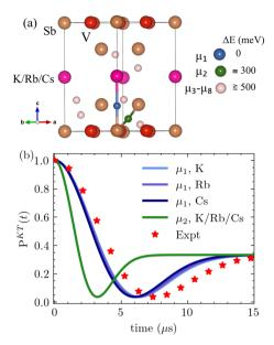
Fig. 6 (a)  $AV_3Sb_5$  (A = K, Rb, Cs) unit cell with eight candidate muon sites, labelled  $\mu_1$  to  $\mu_8$ . (b) Comparison between Kubo-Toyabe polarization function, eqn (1), for the  $\mu_1$  and  $\mu_2$  sites, and the experimental result.83
