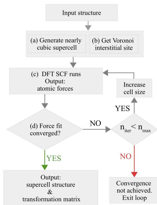
Fig. 2 The flowchart of the supercell convergence workflow implemented in the `IsolatedImpurityWorkChain`. Steps (a)–(d) are described in further detail in the main text.
