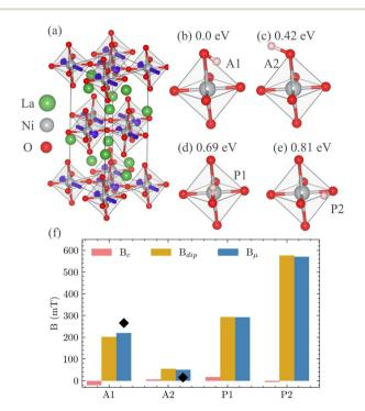
Fig. 8 (a) The magnetic unit cell of La<sub>2</sub>NiO<sub>4</sub>. (b-e) Muon positions (pink spheres) bound to oxygen (labelled A for apical and P for planar) and their relative DFT energies in eV. (f) The contributions to the internal field at the muon in the four sites, where the black diamond symbols indicate reference experimental values.
