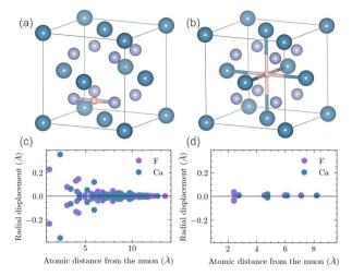
Fig. 7 Muon sites (pink atoms) in CaF<sub>2</sub>: (a) diamagnetic state (Mu<sup>+</sup>) and (b) paramagnetic state (Mu\*). Muon-induced displacements of the host atoms from equilibrium for Mu<sup>+</sup> (c) and for Mu<sup>•</sup> (d).
