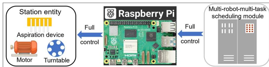
Fig. 10 Control structure for automated experimental stations. The multi-robot–multi-task scheduling module can fully control station operations through Raspberry Pi embedded devices, achieving a high level of automation.
