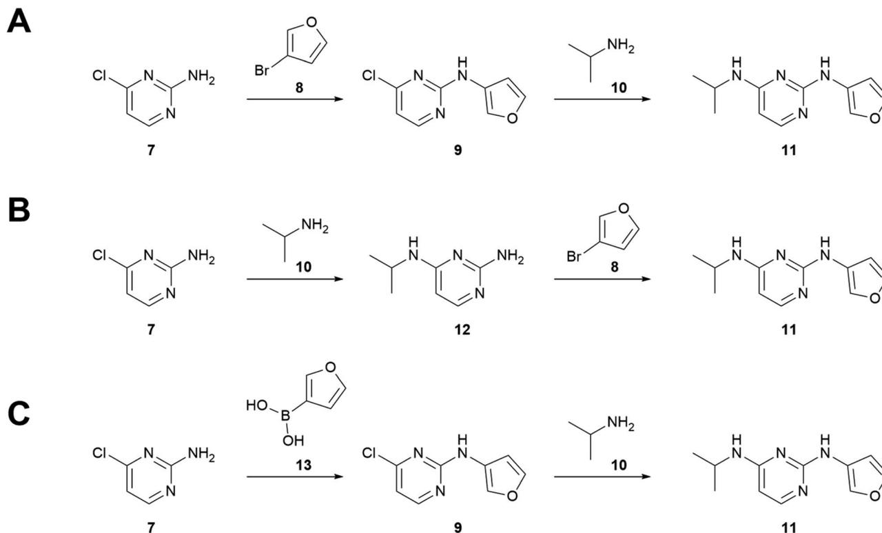
Fig. 2 Three syntheses to make hypothetical pyrimidine **11** starting from **7**. (A) Buchwald–Hartwig,  $S_{\text{N}}\text{Ar}$  sequence. (B)  $S_{\text{N}}\text{Ar}$ , Buchwald–Hartwig sequence. (C) Chan–Lam,  $S_{\text{N}}\text{Ar}$  sequence.  $S_{\text{A,B}} = S_{\text{B,C}} = 0.95$ ;  $S_{\text{A,C}} = 1.0$ .  $\text{TED}_{\text{A,B}} = 4.62$ ;  $\text{TED}_{\text{B,C}} = 4.63$ ;  $\text{TED}_{\text{A,C}} = 1.04$ .
