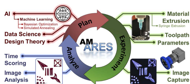
Fig. 3 A simple overview of the closed-loop workflow specific to the Additive Manufacturing (AM) implementation of ARES. Plan: the most up-to-date knowledge base (containing sets of print parameter values and their associated objective scores) is sent via a web server to the planner. Based on the prior knowledge and the specific planner strategy, a subsequent experiment is designed and parameter values are returned to the AM-ARES system. Experiment: the new parameter values are used by AM-ARES to generate machine code that instructs the robot how to print the target geometry. Once complete, the onboard machine vision system captures an image of the printed specimen. Analyze: the AM-ARES system performs analyses based on the human researcher’s analysis selections. The analysis results are then combined with the experimental parameter values and the knowledge base is updated for the next iteration.
