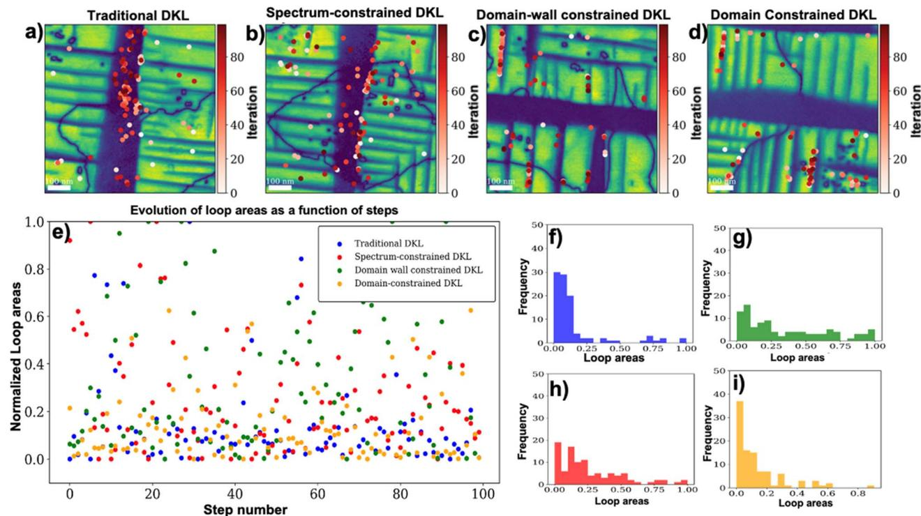
Fig. 7 Constrained DKL in operating autonomous microscopy. (a)–(d) Sampled BEPS measurement locations of traditional DKL, spectrum constrained DKL, domain wall constrained DKL, and domain constrained DKL, respectively. (e) Hysteresis loop area as a function of DKL exploration steps. (f–i) Histograms of loop area distribution 1 of traditional DKL, spectrum constrained DKL, domain wall constrained DKL, and domain constrained DKL, respectively.
