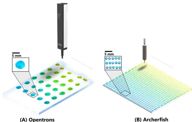
Fig. 5 Combinatorial printing throughput comparison between Opentrons and Archerfish. (A) Opentrons printing of colored dyes at a rate of 2.5 unique compositions per minute with *ex situ* mixing and stepwise printing. (B) Archerfish printing of colored dyes at a rate of 250 unique compositions per minute with *in situ* mixing and continuous printing.
