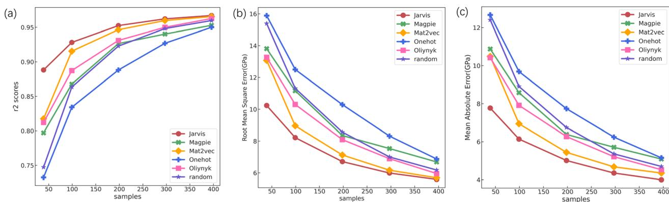
Fig. 3 The performance of predicting the bulk modulus, using 6 CBFV descriptors—Jarvis, Magpie, Mat2vec, Onehot, Oliylyk, and random—within RF models, evaluated on training data (495 carbides, including 9 monocarbides, 108 binary carbides, 252 ternary carbides, and 126 equimolar quaternary HECs) (a) the predicted  $R^2$ ; (b) the predicted RMSE; (c) the predicted MAE.
