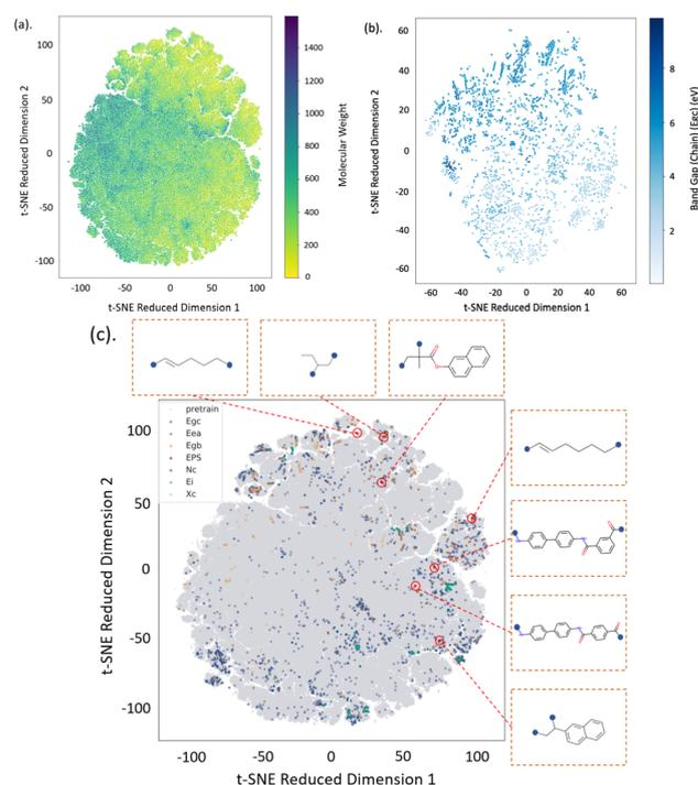
**Fig. 5** t-SNE dimensional reduction analysis of the polymer representation space learnt by PolyCL. Visualisation of the continuous representation of polymer repeating units: (a) The unsupervised pre-trained dataset coloured by molecular weight; (b) The  $E_{\text{gc}}$  dataset coloured by the band gap (chain) property and (c) all available datasets coloured by the data origin, with selected polymers shown. The blue dot denotes the connection point of the repeating unit to the polymer chain.
