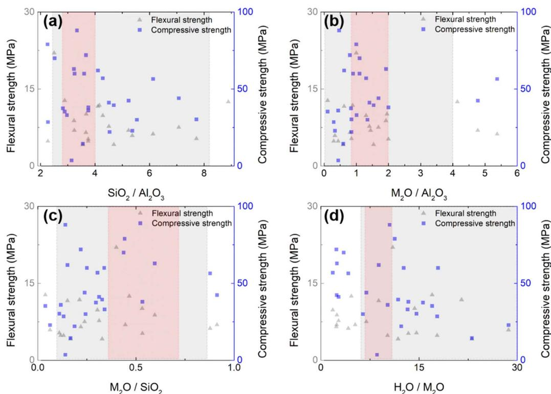
Fig. 3 Flexural strength and compressive strength values according to the ratio of synthetic raw materials, including alkali activator and binder: (a)  $\text{SiO}_2/\text{Al}_2\text{O}_3$ , (c)  $\text{Na}_2\text{O}/\text{SiO}_2$ , (b)  $\text{Na}_2\text{O}/\text{Al}_2\text{O}_3$ , and (d)  $\text{H}_2\text{O}/\text{Na}_2\text{O}$ . The shaded grey area represents the range of our preliminary tests based on literature, while the red area represents the range explored in the DOEs of this study.
