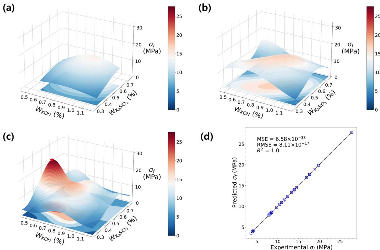
Fig. 4 The RBF models for flexural strength of GPs with  $\text{H}_2\text{O}$  fixed at 0. The development of the RBF model as DOE sets proceed: with the accumulated dataset of (a)  $\text{D}_1$  only, (b)  $\text{D}_1$  and  $\text{D}_2$ , and (c)  $\text{D}_1$ – $\text{D}_3$ . (d) The parity plot shows the distribution of experimental vs. predicted flexural strength, with the  $y = x$  line represented by dashed lines. The RBF model is fitted with  $R^2 = 1.0$ .
