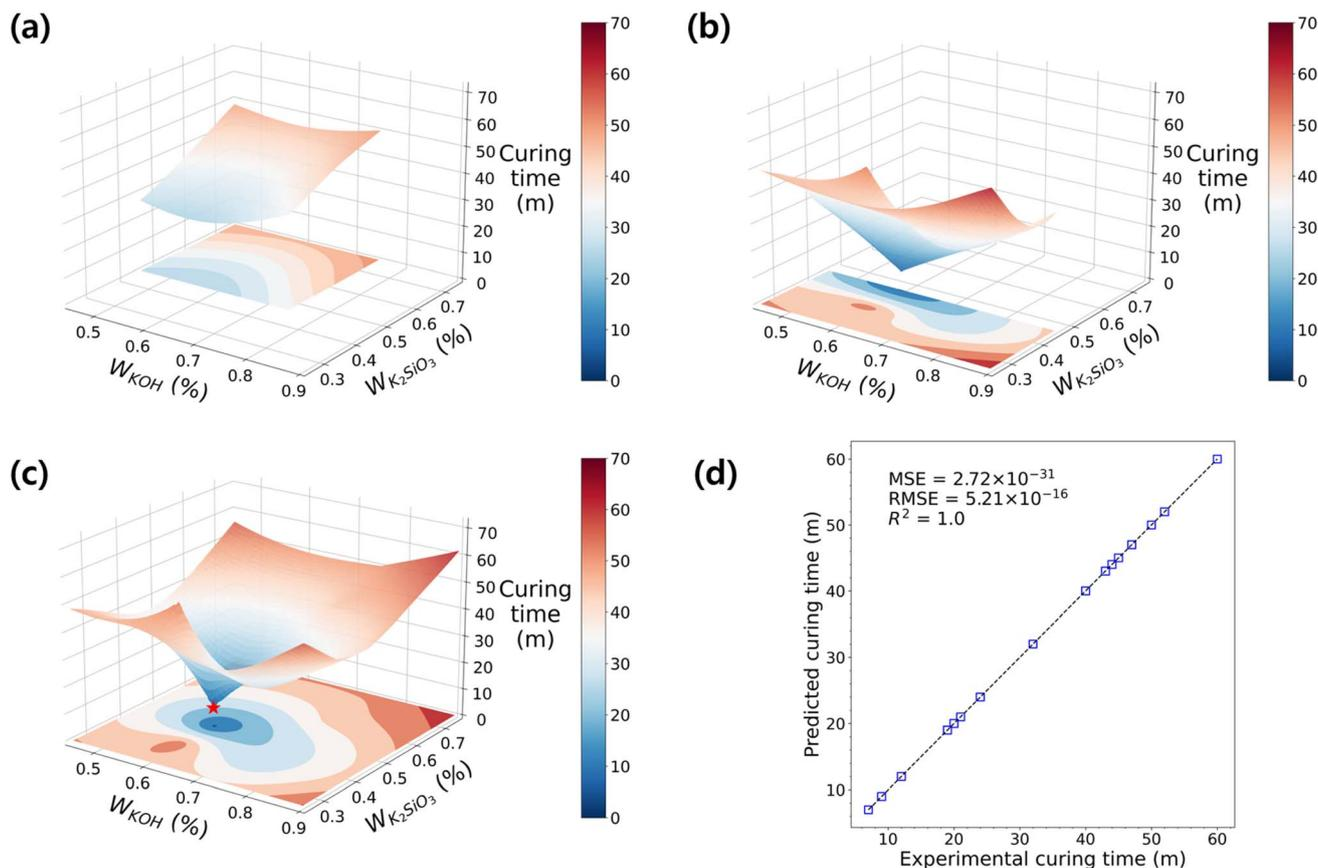
Fig. 5 The RBF models for curing time of GPs with  $\text{H}_2\text{O}$  fixed at 0. The development of the RBF model as DOE sets proceed: with the accumulated dataset of (a)  $\text{D}_2$  only, (b)  $\text{D}_3$  only, and (c)  $\text{D}_2$  and  $\text{D}_3$ . (d) The parity plot shows the distribution of experimental vs. predicted curing time, with the  $y = x$  line represented by dashed lines. The RBF model is fitted with  $R^2 = 1.0$ .
