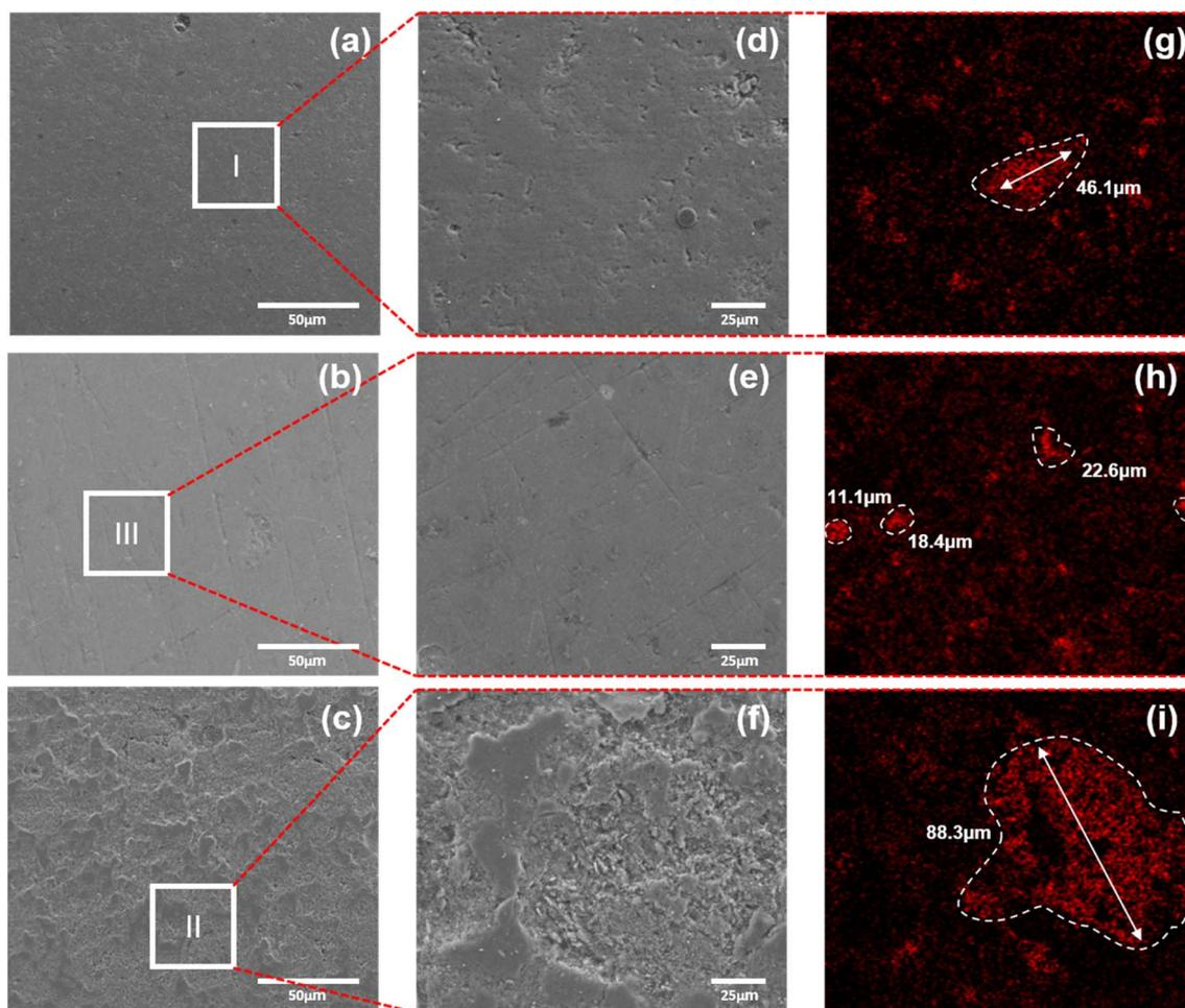
Fig. 7 (a–f) Cross-sectional images and (g–i) EDS analysis of geopolymers: (I) GP<sub>IFC</sub>, (II) GP<sub>OFC</sub> and (III) GP<sub>OC</sub>. (a–c) and (d–f) show surfaces at different magnifications. In (g–i), Ca elements are indicated in red, and the size of Ca compounds is estimated.
