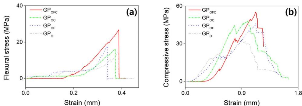
Fig. 6 Representative stress–strain curves of GP<sub>OFC</sub> (red), GP<sub>OC</sub> (green), GP<sub>OF</sub> (blue), and GP<sub>O</sub> (gray) for (a) flexural test and (b) compressive test.
