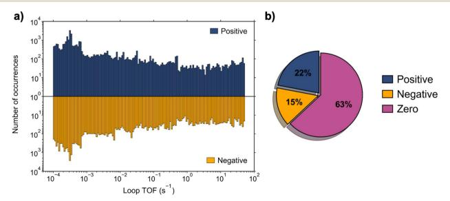
Fig. 2 Complete three-species loop simulation dataset. (a) Simulations that returned a non-zero loop TOF ranged in magnitude from  $10^{-4}$  to 50 $s^{-1}$ . Most simulations exhibited lower magnitudes of loop TOF,  $<10^{-2}$  s<sup>-1</sup>. (b) Nearly two-thirds of the output loop turnover frequency values were zero, defined as having magnitude less than  $10^{-4}$  s<sup>-1</sup>, with slightly more of the non-zero simulations having positive loop TOF.
