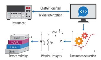
Fig. 1 Diagram depicting the Al-engineered current-voltage (IV) characterization module and parameter extraction tool described in this work. The Source Measure Unit (SMU) is connected to a control computer running a Python application developed by ChatGPT. The collected IV characterization data is subsequently processed using a high-performance differential evolution algorithm for automated parameter extraction from the IV curves, to provide insights for redesigning the device stack.
