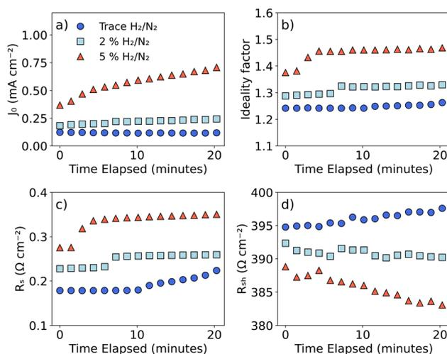
Fig. 7 Single-diode parameters as a function of time and forming gas percentage in the  $N_2 + H_2/N_2$  mixture for the tested Cr<sub>2</sub>O<sub>3</sub>/β-Ga<sub>2</sub>O<sub>3</sub>-based heterojunction diode. Device degradation was observed upon exposure to  $H_2/N_2$  while enduring a temperature soak at  $500$  °C.
