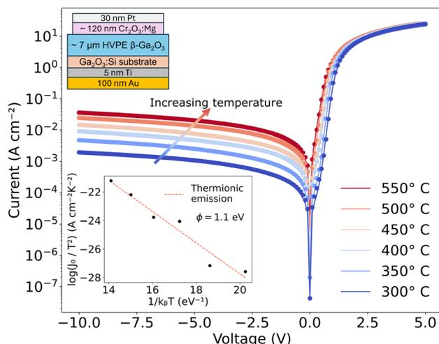
Fig. 6 Architecture of a Pt/Cr<sub>2</sub>O<sub>3</sub>:Mg/β-Ga<sub>2</sub>O<sub>3</sub>-based heterojunction diode and corresponding current–voltage data measured at several temperatures. Points represent experimental data and the solid lines represent the fits with the best set of single diode parameters that models the data. MAPEs for ranged between 4.7% and 7.8%. The inset shows that  $J_0$  can be modelled by the thermionic emission model, yielding a barrier height of 1.1 eV.
