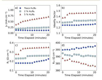
Fig. 7 Single-diode parameters as a function of time and forming gas percentage in the  $N_2 + H_2/N_2$  mixture for the tested  $Cr_2O_3/\beta$ - $Ga_2O_3$ based heterojunction diode. Device degradation was observed upon exposure to H<sub>2</sub>/N<sub>2</sub> while enduring a temperature soak at 500 °C.
