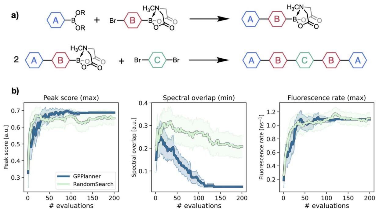
Fig. 5 (a) Reaction scheme of iterative Suzuki–Miyaura cross-coupling reaction proposed to synthesize symmetric A–B–C–B–A pentamers in the `dye_lasers` dataset. (b) Individual objective traces corresponding to the experiment with the best hypervolume value as a function of the number of transpired experiments. Solid lines represent the mean objective values averaged over 50 independent runs and shaded regions represent the 95% confidence interval.
