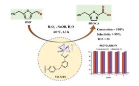
Supported vanadium- and tungsten-based catalysts for selective and sustainable oxidation of 5-hydroxymethylfurfural to 5-hydroxymethyl-2furancarboxylic acid with H2O2 in water
