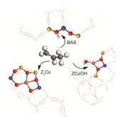
Unraveling the C<sub>3</sub>H<sub>6</sub> poisoning mechanism of Z<sub>2</sub>Cu and ZCuOH sites over Cu-SSZ-13 during NH<sub>3</sub>-SCR
