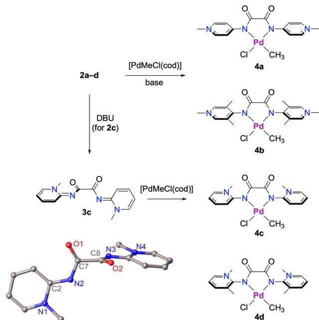
**Scheme 2** Synthesis of Pd complexes **4a–4d** with PYA ligand sites represented in their zwitterionic (pyridinium amidate) resonance form, though there is also contribution from a neutral pyridylidene imine resonance form to be considered. Bottom left: crystallographically determined molecular structure of **3c** (50% probability ellipsoids, hydrogen atoms omitted for clarity). Selected metrics for **3c**: N2–C2 1.338(14) Å; C7–N2–C2–N1 4.01(9)°.
