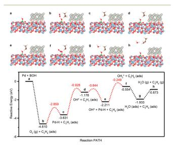
Fig. 5 DFT calculated energy profile for ODHP over Pd-B/Al<sub>2</sub>O<sub>3</sub> following a surface-catalyzed pathway. The diagram presents the energy profile along the reaction coordinate, highlighting the initial state, transition state, and final state from left to right. The models (ah) show side views of the geometries for the various states. The atoms are color-coded as follows: Pd in grey, B in green, Al in light blue, O in red, C in dark brown, and H in pink.
