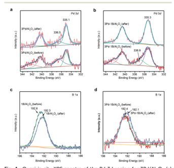
Fig. 4 Quasi in situ XPS spectra of the Pd 3d region for  $3Pd/Al_2O_3$  (a) and  $3Pd-1B/Al_2O_3$  (b), and the B 1s region for  $1B/Al_2O_3$  (c) and  $3Pd-1B/Al_2O_3$  (d), recorded before and after ODHP reaction for 1 h.
