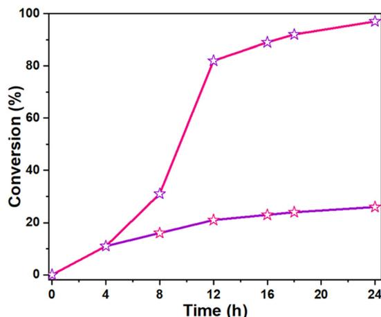
Fig. 6 Plot of conversion (%) versus time for the **Zn-(p-GluBenz)** catalyst. The purple line represents the reaction progress after catalyst removal at 4 h, while the pink line shows product conversion over 24 h with the catalyst present.
