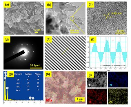
Fig. 2 (a) FESEM image, (b) TEM image, (c) HRTEM image, (d) selected area electron diffraction pattern, (e) lattice fringes, (f) average *d*-spacing, (g) energy dispersive X-ray (EDX) elemental spectrum with composition results, and (h and i) elemental mapping images of **Zn**-(p-**GluBenz**).
