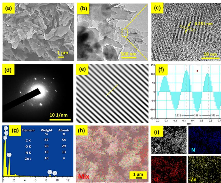
Fig. 2 (a) FESEM image, (b) TEM image, (c) HRTEM image, (d) selected area electron diffraction pattern, (e) lattice fringes, (f) average *d*-spacing, (g) energy dispersive X-ray (EDX) elemental spectrum with composition results, and (h and i) elemental mapping images of **Zn-(D-GluBenz)**.
