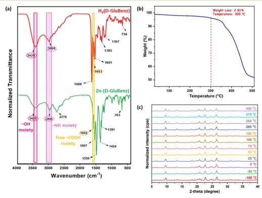
Fig. 1 (a) Comparison of FTIR spectra of  $H_3(D-GluBenz)$  and Zn-(D-GluBenz), highlighting the catalytic sites, (b) thermogravimetric analysis profile and (c) VT PXRD patterns from -100 to +300 °C of Zn-(D-GluBenz).
