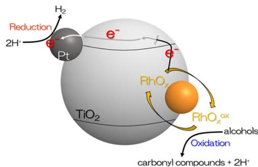
**Fig. 7** Expected reaction mechanism for formation of H<sub>2</sub> and carbonyl compounds from various alcohols over RhO<sub>x</sub>/TiO<sub>2</sub>–Pt photocatalyst under irradiation of visible light.
