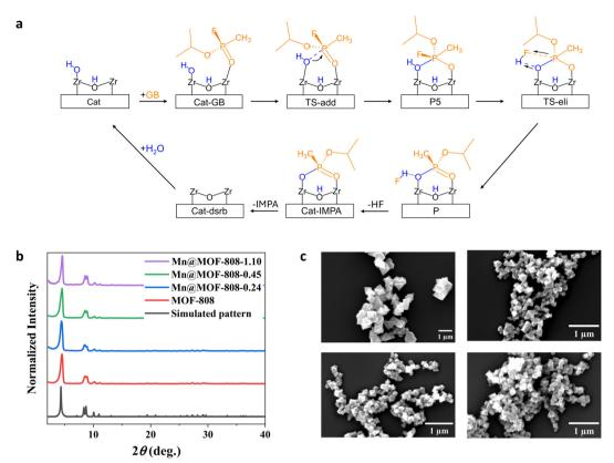
Fig. 1 (a) Reaction mechanism for the hydrolysis of sarin (GB) on native MOF-808. (b) PXRD patterns and (c) SEM images of i) MOF-808, ii) Mn@MOF-808-0.24, iii) Mn@MOF-808-0.45, and iv) Mn@MOF-808-1.10.
