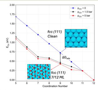
Fig. 2  $E_{Co}$  scaling with CN with increasing  $p_{CO}$
