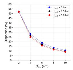
Fig. 5 Dispersion (defined as  $N_{\text{surf}}/N_{\text{tot}}$  where  $N_{\text{tot}}$  and  $N_{\text{surf}}$  are the total number of atoms and number of surface atoms, respectively) of free-standing Co NPs with increasing  $D_{Co}$  and  $p_{CO}$ . Error bars have been omitted as they are negligibly small.
