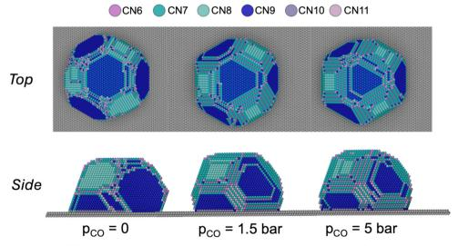
Fig. 4 Top and side views of a CoTiO<sub>3</sub>-supported 8 nm Co NP in vacuum, in the high  $X_{CO}$  ( $p_{CO} = 1.5$  bar) and low  $X_{CO}$  ( $p_{CO} = 5$  bar) scenarios. Co atoms are colored based on their coordination number.
