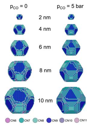
Fig. 3 Structural models of Co NPs in the investigated size range in vacuum and exposed to  $p_{CO} = 5$  bar.
