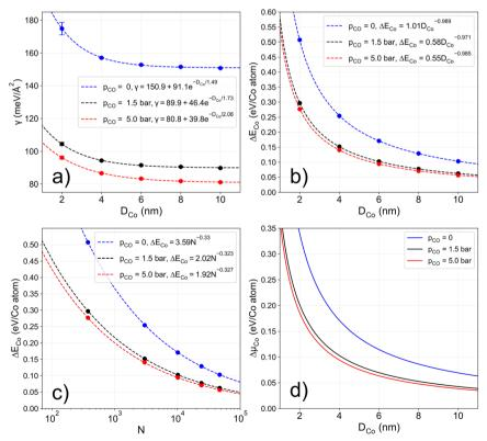
Fig. 7 Free-standing Co NPs a) surface energies with increasing  $D_{Co}$  and  $p_{CO}$ , b) average energy per atom  $\Delta E_{Co}$  with respect to bulk Co with increasing  $D_{Co}$  and  $p_{CO}$  and c) with increasing number of atoms (N) and  $p_{CO}$ . d) Chemical potential of the free-standing Co NPs in respect to bulk Co  $\Delta\mu_{Co}$  with increasing  $D_{Co}$  and  $p_{CO}$ .
