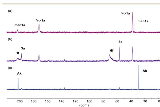
**Fig. 6** <sup>31</sup>P{<sup>1</sup>H} NMR (202 MHz, toluene-*d*<sub>8</sub>): spectra of **1a** (a), activated **1a** by reaction with H<sub>2</sub> and KO<sup>t</sup>Bu after 15 min sonication (b), reaction of the latter with benzophenone (5 equiv., c).
