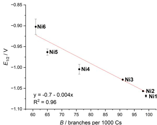
**Fig. 5** Plot of experimentally determined  $E_{1/2}$  values (in V) against the experimental branching density  $B$  ( $R^2 = 0.96$ ).
