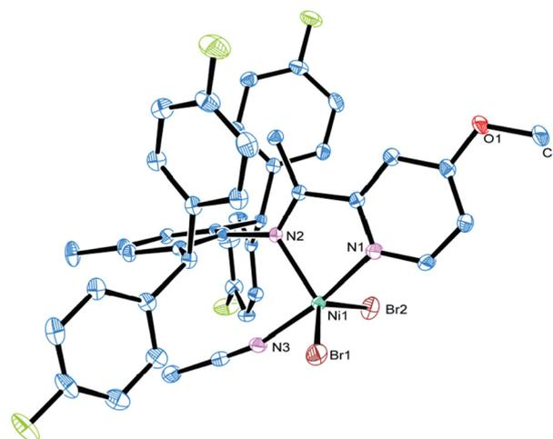
**Fig. 1** ORTEP representation of Ni1(NCMe) with the thermal ellipsoids set at the 50% probability level; the hydrogen atoms have been omitted for clarity. Selected bond distances (Å): Ni(1)–Br(1) 2.4506(4), Ni(1)–Br(2) 2.4538(5), Ni(1)–N(1) 2.0255(19), Ni(1)–N(2) 2.0465(18), Ni(1)–N(3) 2.0373(19), selected bond angles (°): Br(1)–Ni(1)–Br(2) 135.581(18), N(1)–Ni(1)–Br(1) 90.21(6), N(1)–Ni(1)–Br(2) 89.37(6), N(1)–Ni(1)–N(2) 78.98(7), N(1)–Ni(1)–N(3) 171.33(8).
