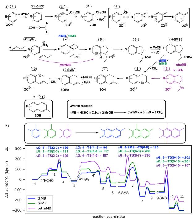
Fig. 2 a) Reaction scheme of the investigated naphthalene formation mechanism. -R = dimethyl, trimethyl, tetramethyl, nMB = n-methylbenzene, (n + 1). MN = (n + 1)-methylnaphthalene. b) Investigated isomers of reactants and products. c) Gibbs free energy diagrams of reaction free energies for naphthalene formation with di-, tri- and tetramethylbenzene. Reaction barrier heights are indicated above the respective barriers. Reaction temperature is 400 °C; reference pressure = 1 bar.
