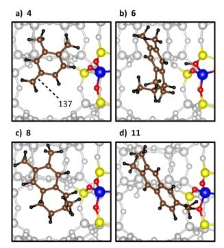
4 Structures of important intermediates in the naphthalene formation process starting from dimethylbenzene. Color code: blue: Al, yellow: Si, red: O, brown: C, black: H. Bond lengths indicated in pm.
