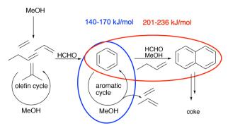
Fig. 6 Placing the results of this work (highlighted in red) in the context of MTO reactions. Reaction barriers for ethylene and propylene formation (highlighted in blue) are taken from ref. 69 and ref. 70.
