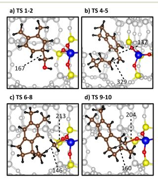
Fig. 3 Structures of important transition states in the naphthalene formation process starting from dimethylbenzene. Color code: blue: Al, yellow: Si, red: O, brown: C, black: H. Bond lengths indicated in pm.
