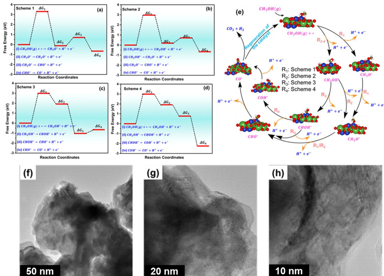
Fig. 6 Schematic representation of the (a)–(e) free energy diagram for the MOR using different mechanistic schemes. The \* represents the active surface of the LCO catalyst. (f)–(h) HRTEM image of the LCO catalyst at different resolutions. Color code: red: oxygen, green: lanthanum, grey: nickel, blue: copper, black: zinc, white: hydrogen, and brown: carbon.
