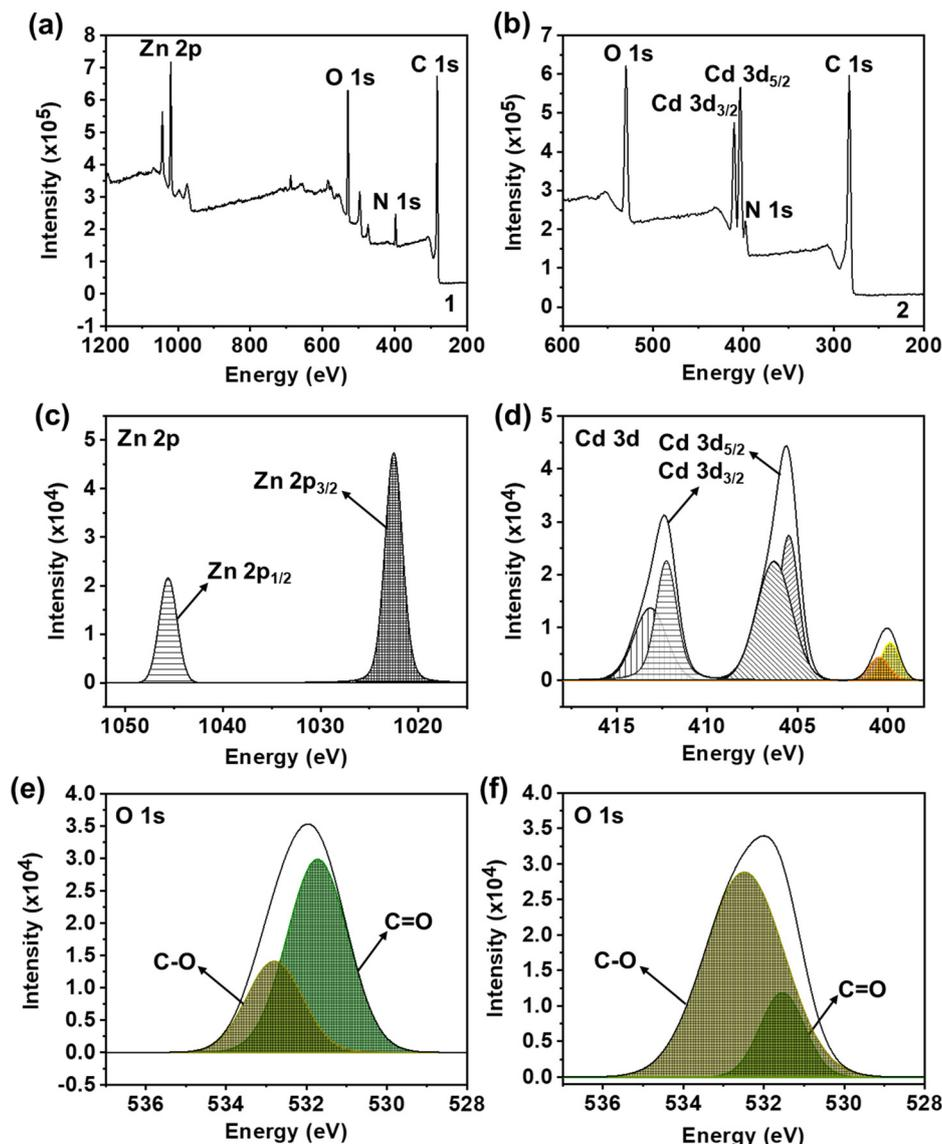
Fig. 4 (a and b) Full range XPS spectra of **1** and **2**, respectively. (c and d) Deconvoluted XPS spectra of Zn 2p and Cd 3d in **1** and **2**, respectively. (e and f) Deconvoluted XPS spectra of O 1s in **1** and **2**, respectively.
