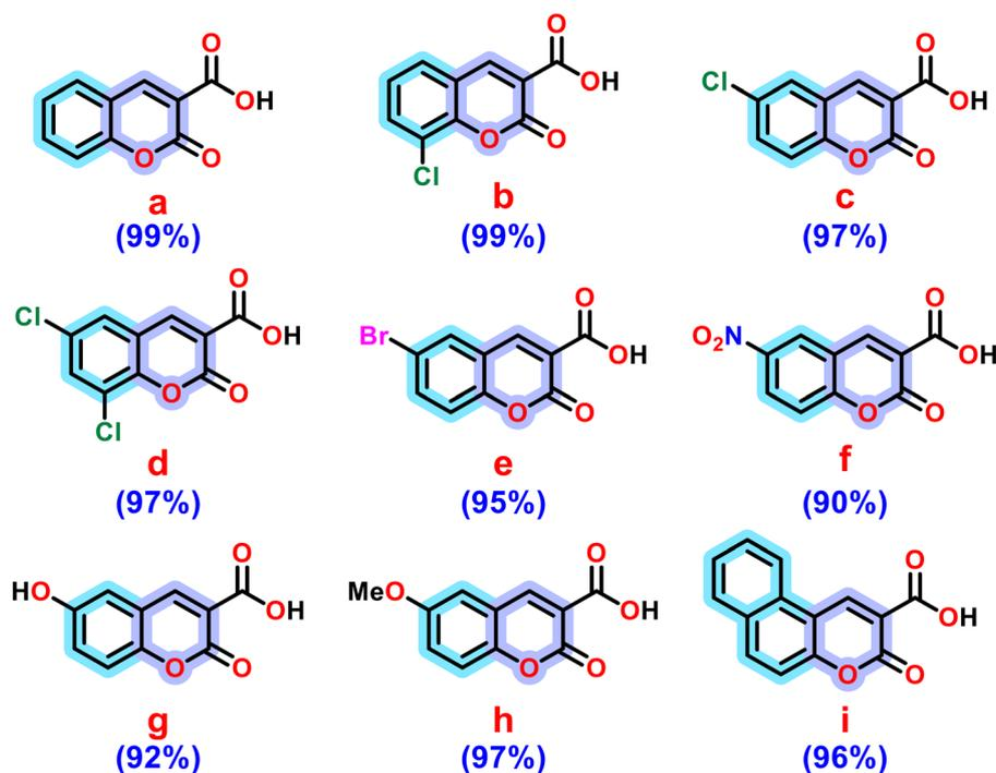
**Scheme 3** Substrate scope with conditions used: derivatives of salicylaldehyde (0.1 mmol), Meldrum's acid (0.15 mmol), and **2** (1.5 mol%) at 25 °C in methanol. Numbers in parentheses are the isolated yields (%) of C-3-CAs.
