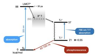
Fig. 4 Jablonski-type diagram summarizing the known information about the excited states of DT. Given various reports on the picosecond dynamics of the system, we speculate that a state,  $X^*$  may be involved in HAT from water and possibly in the path to  $^3DT^*$ .
