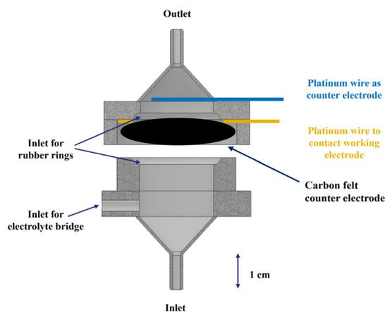
**Fig. 1** Flow-through reaction cell with coated carbon felt as a working electrode, in contact circularly all around. The counter electrode is a platinum wire and a reference Ag/AgCl electrode is connected *via* an electrolyte bridge inserted through an inlet. Rubber rings are included for sealing.
